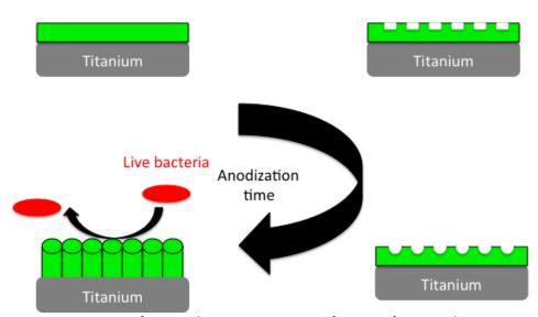
**Scheme 3:** Formation process of nanotubes on titanium surfaces. Before anodization, a nanoscale  $TiO_2$  passivation layer is present on Ti surfaces and whenever a constant voltage is applied, pits are formed on the  $TiO_2$  layer. As anodization time increases, pits grow longer and larger resulting in nanopore formation. After a specific anodization time, nanotubes are formed on the Ti surface.
