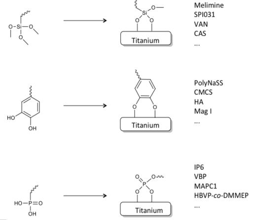
**Scheme 2:** A selection of anchors on titanium surfaces with different functionalizations to achieve an antimicrobial surface.
