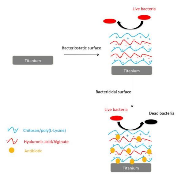
**Scheme 4:** Layer by layer coating of polycationic and polyanionic polymers to make bacteriostatic surfaces. Then, thanks to the introduction of an antibiotic, titanium surfaces become both bacteriostatic and bactericidal.
