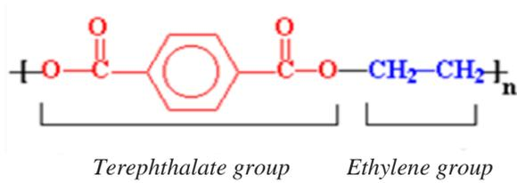
Fig. 1. Chemical formula of Poly(Ethylene Terephthalate)
