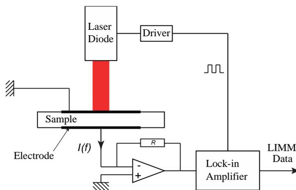
Fig. 2. Schematic of the L IMM set-up
