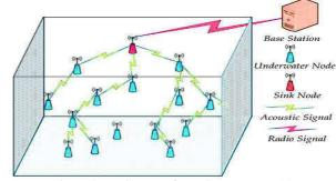
Figure 13. Deployment of an underwater WSN [34]
