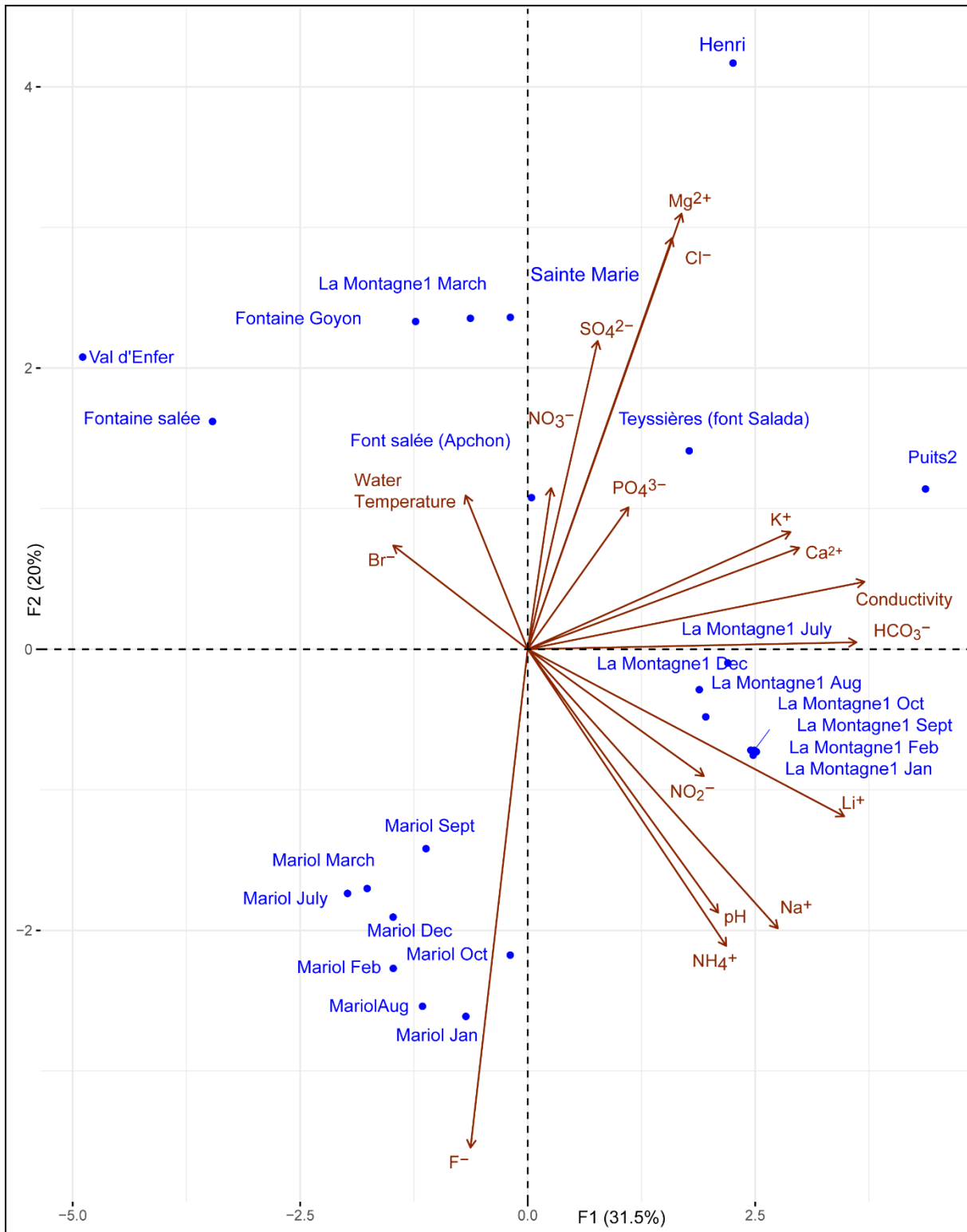
Figure 9. First factorial plan of the Principal Component Analysis done on the springs and their physical and chemical composition.
