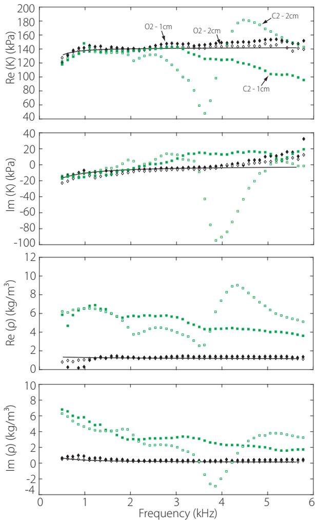
FIG. 4. Effective acoustic longitudinal modulus  $K$  and density  $\rho$  as functions of frequency for the small pores foams. Results for open-cell foams are shown in black symbols, while that for closed-cell ones are in green. Two thicknesses are shown: 2 cm (open symbols) and 1 cm (solid symbols). Solid black lines show JCAL model for the open-cell foam O2.
