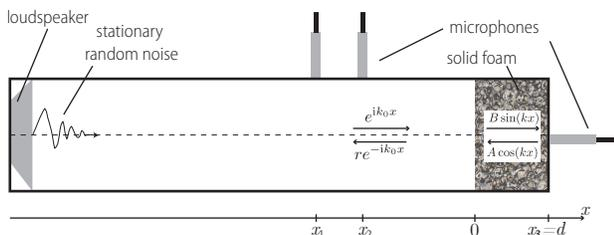
FIG. 2. Impedance tube mounted with two microphones in reflection and one in transmission. Characteristic parameters of the tube :  $x_1 = -14.5$  cm,  $x_2 = -12.5$  cm,  $x_3 = +2$  cm (or +1 cm), diameter of the tube was 29 mm.
