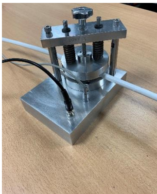
Fig. 4: PEA cell for space charge measurement for aeronautical DC cables.
