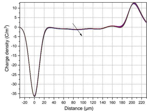
b) Sample after Gamma irradiation 60 kGy. Volt ON
