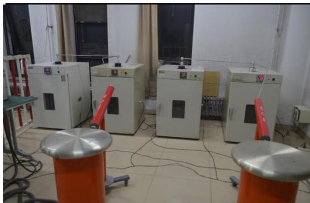
**Figure 4.** Picture of thermo-electric aging system.
