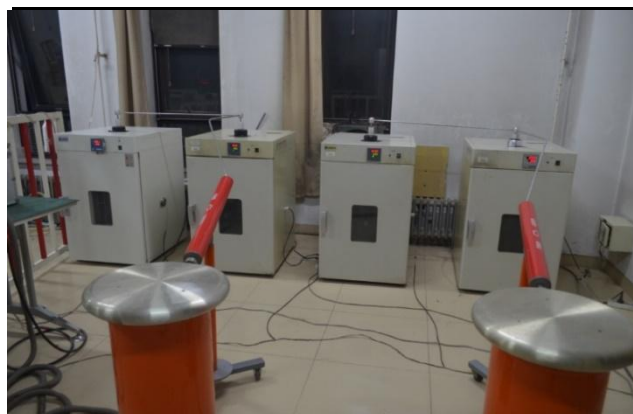
Figure 4. Picture of thermo-electric aging system.
