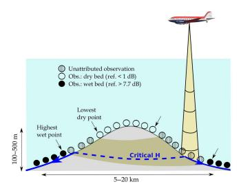
**Figure 2.** This figure illustrates how water and basal topography are linked with a region of flat surface for a uniform local GF. The blue line shows the presence of water at the bed and the direction of its flow. The brown area corresponds to a strip where the thermal conditions are unknown. We defined the critical thickness as the minimum thickness that allows basal melting today.
