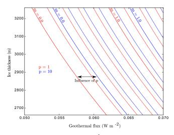
Figure 6. Basal melt rate m in mm a<sup>-1</sup>, depending on the ice thickness, GF and shape parameter p.
