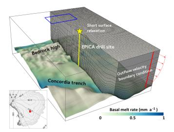
**Figure 1.** Mesh, bedrock dataset (Fretwell et al., 2013; Young et al., 2017) and basal melt rate (Passalacqua et al., 2017) used for the simulation on a  $83 \times 114$  km domain. The red patch on the context map (bottom left) shows the domain used for the calculation, and the blue rectangle at the top of the image is the location of Fig. 2.
