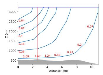
**Figure 3.** Trajectories of the ice particles from the ice surface towards the black point in Fig. 2 (dashed red trajectory). Red numbers indicate the age of the ice, in millions of years. The bed profile is shown in grey. The thin red line corresponds to one possible drill site (red point in Fig. 2).
