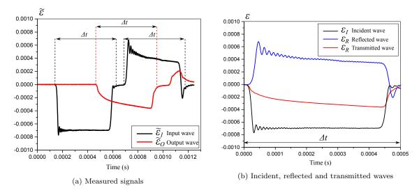
Fig. 2: Wave measurements
