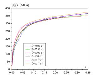
Fig. 7: Material variability and independence on strain-rate
