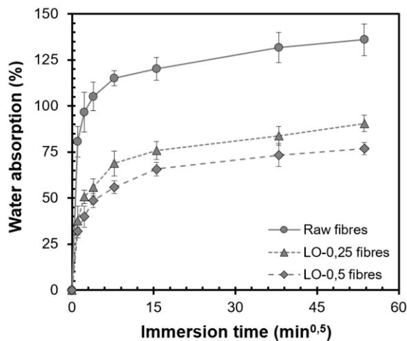
Fig. 6: Water absorption of raw and treated flax fibres.
