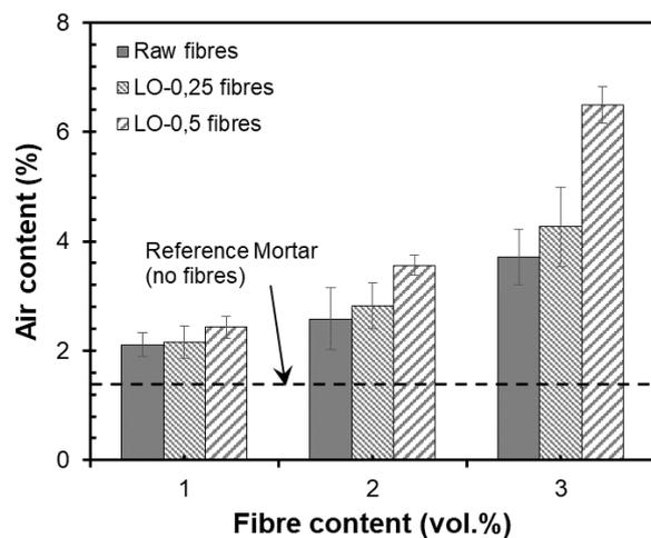
Fig. 7: Estimated air content of fresh mortars.
