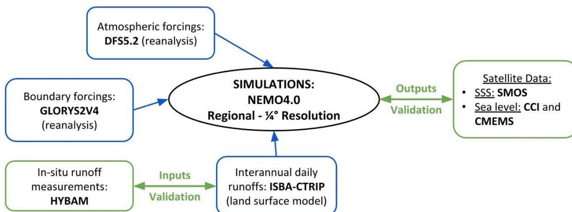
Figure 1. Model configuration and data used for validation.
