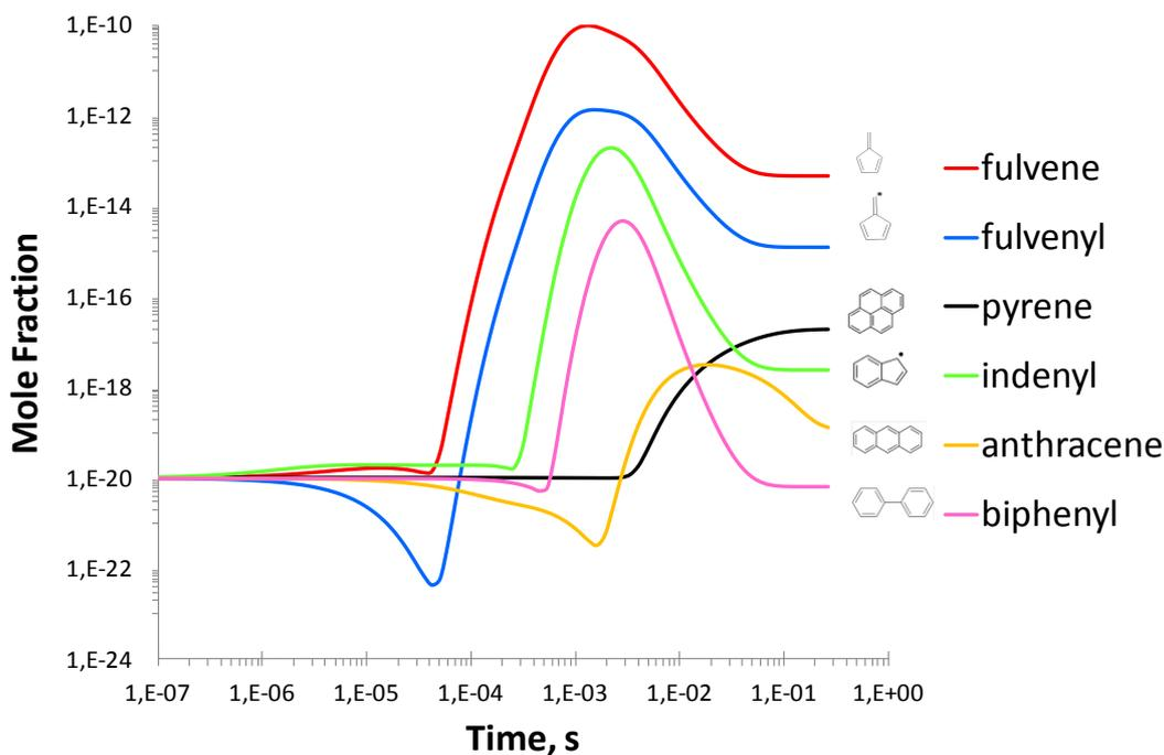
**Figure 14.** Time evolution of polycyclic aromatic hydrocarbons (PAHs) carbon species calculated from Table 3, OPT 1 conditions.  $T_s=700^\circ\text{C}$ ,  $P=13$  mbar,  $\Phi_{\text{CH}_4}=1$  sccm,  $\Phi_{\text{H}_2}=50$  sccm and  $P_{\text{mw}}=400$  W.
