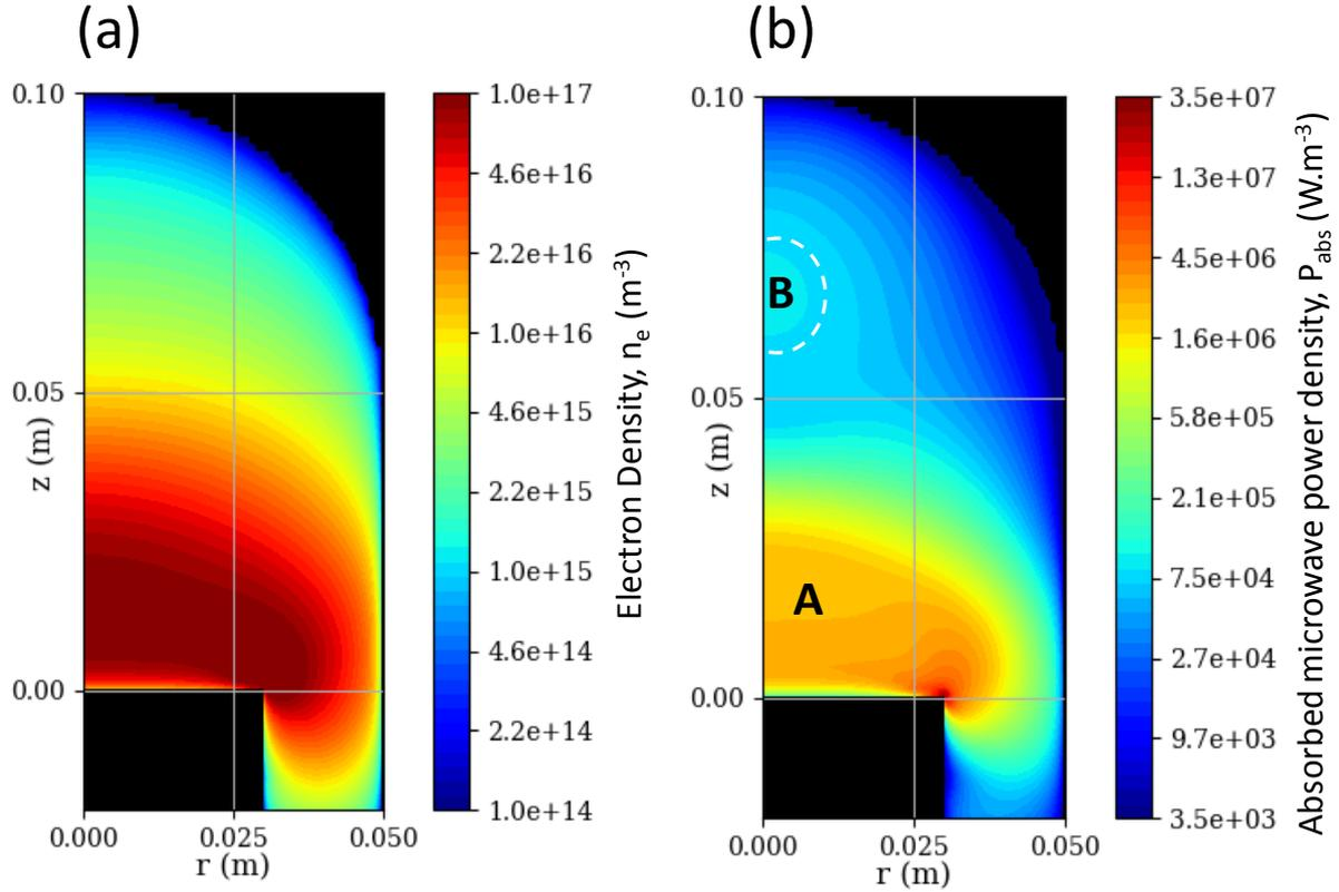
**Figure 17.** (a) Electron density and (b) absorbed power density contours. Calculated from Table 3, OPT 3 conditions.  $z$  and  $r$  are axial and radial position in meters, respectively.  $T_s=870^\circ\text{C}$ ,  $P=13$  mbar,  $\Phi_{\text{CH}_4}=1$  sccm,  $\Phi_{\text{H}_2}=50$  sccm and  $P_{\text{mw}}=400$  W.
