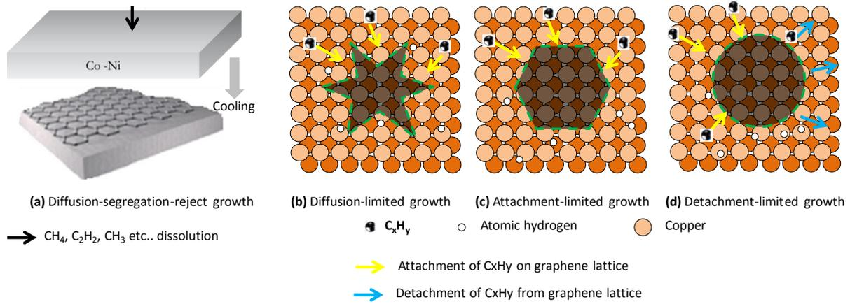
**Figure 20.** Schematics of graphene growth on (a) low carbon solubility cobalt substrate and (b-c) high carbon solubility copper substrate at different substrate temperature.
