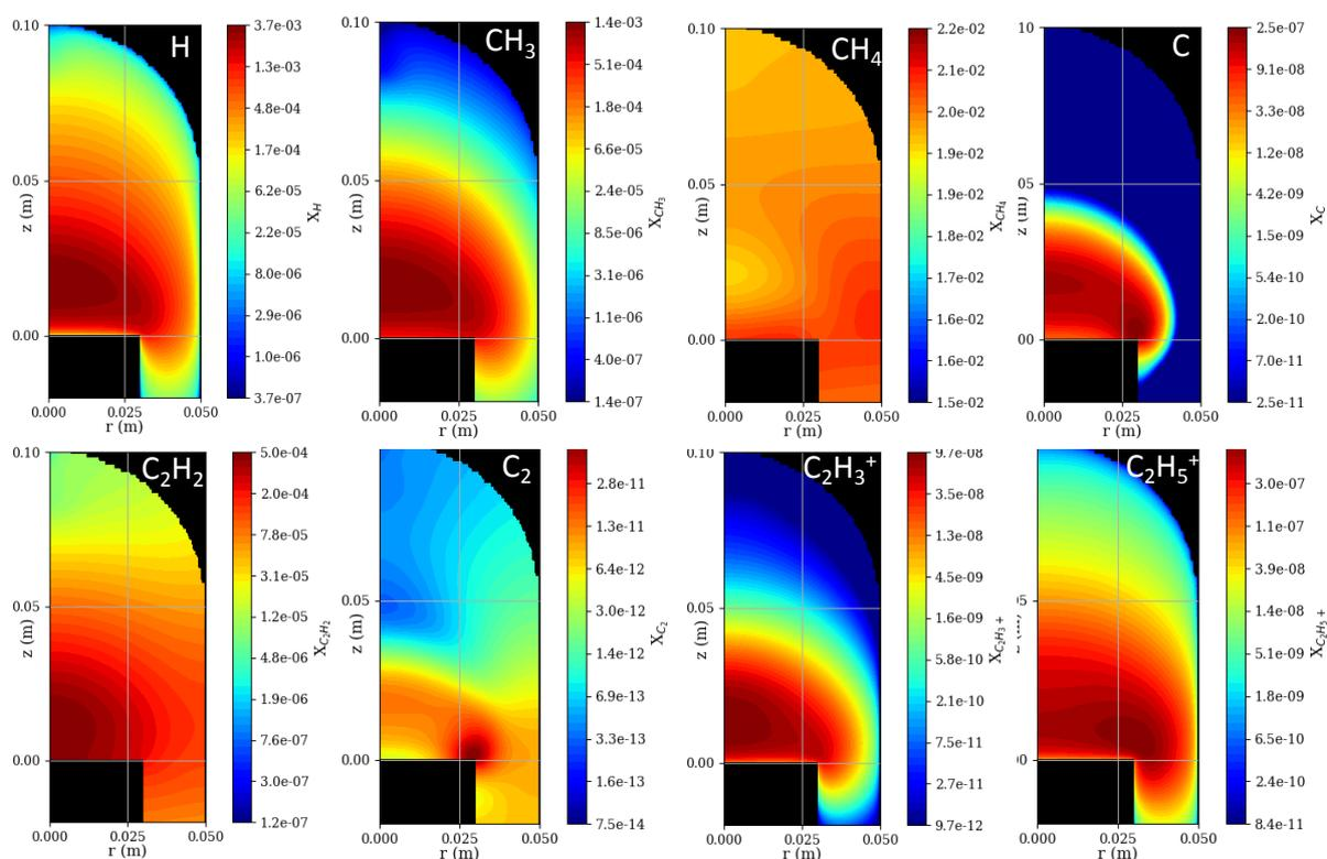
**Figure 18.** Specie mole fraction contours for H, CH<sub>3</sub>, CH<sub>4</sub>, C (Top from left to right) and C<sub>2</sub>H<sub>2</sub>, C<sub>2</sub>, C<sub>2</sub>H<sub>3</sub><sup>+</sup> and C<sub>2</sub>H<sub>5</sub><sup>+</sup> (Bottom from left to right) calculated from Table 3, OPT 3 conditions. z and r are axial and radial position in meters, respectively. Ts=870°C, P=13 mbar,  $\Phi_{CH_4}$ =1 sccm,  $\Phi_{H_2}$ =50 sccm and P<sub>mw</sub>=400 W.
