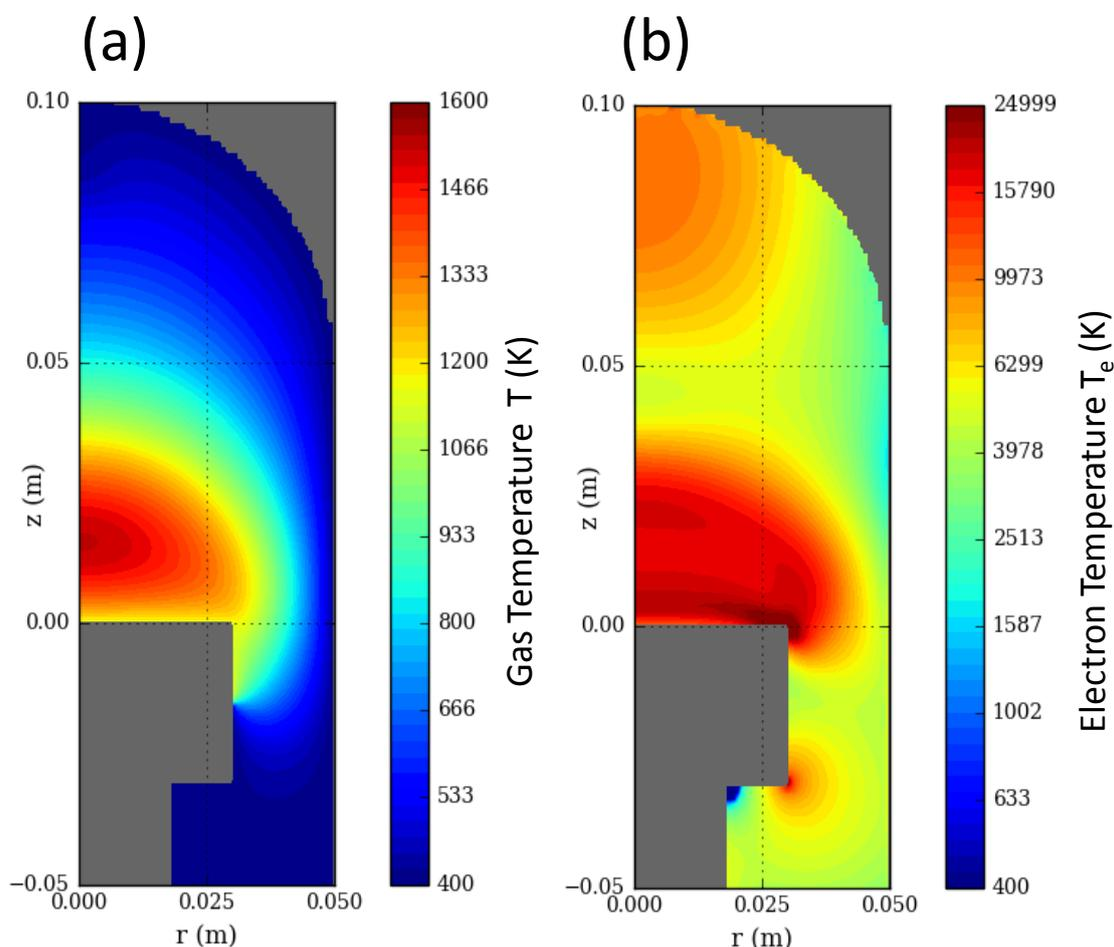
**Figure 16.** Contours of (a) gas temperature  $T$  and (b) electron temperature  $T_e$  calculated from Table 3, OPT 3 conditions.  $z$  and  $r$  are axial and radial position in meters, respectively
