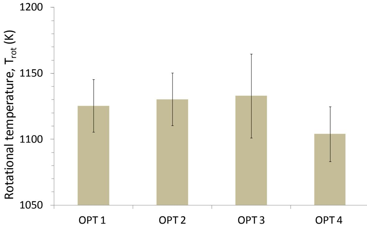
**Figure 7.** H<sub>2</sub> rotational temperature measured by OES at the optimal graphene growth conditions of Table 3.
