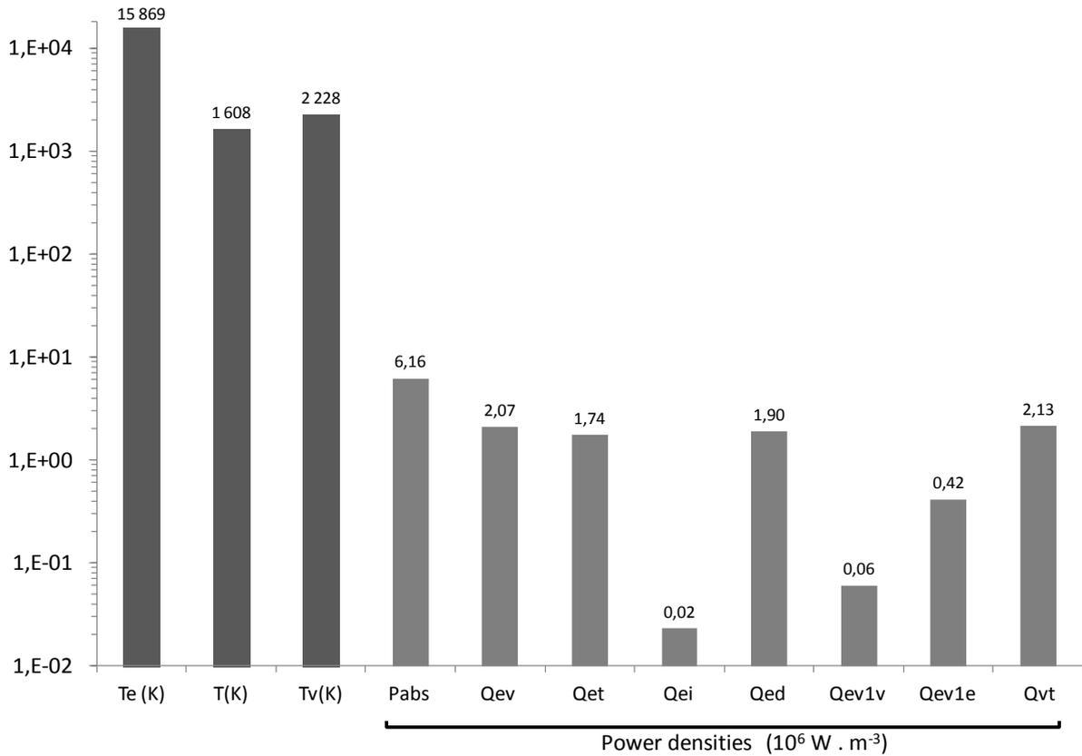
**Figure 15.** Electron, gas and vibration temperatures, absorbed power and electron and vibration energy exchange calculated for OPT 1 conditions.  $T_s=700^\circ\text{C}$ ,  $P=13$  mbar,  $\Phi_{\text{CH}_4}=1$  sccm,  $\Phi_{\text{H}_2}=50$  sccm and  $P_{\text{mw}}=400$  W.
