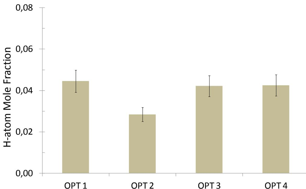
**Figure 10.** Atomic hydrogen mole fraction as determined from actinometry in the optimal graphene growth conditions of Table 3.
