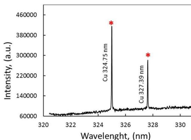
**Figure 8.** Copper lines observed from emission spectrum in pure hydrogen when copper catalyst is used.
