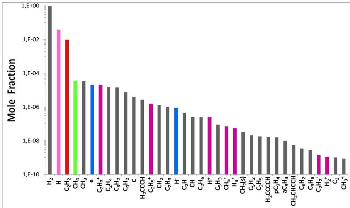
**Figure 12.** Major species calculated from Table 3, OPT 1 conditions.  $T_s=700^\circ\text{C}$ ,  $P=13$  mbar,  $\Phi_{\text{CH}_4}=1$  sccm,  $\Phi_{\text{H}_2}=50$  sccm and  $P_{\text{mw}}=400$  W.
