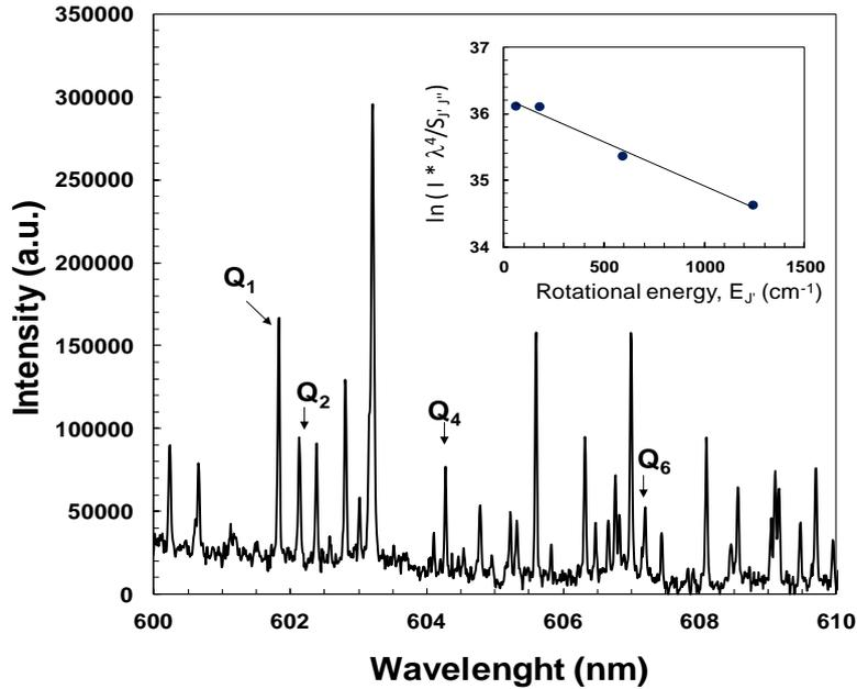
**Figure 5.** Example of measured H<sub>2</sub> Fulcher- $\alpha$  Q-branch spectrum with indication to the selected rotational lines at microwave power of 390 W and total pressure of 13 mbar. The inset shows the corresponding Boltzmann plot.
