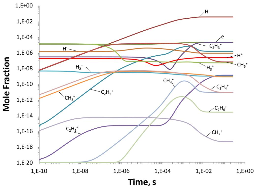
**Figure 13.** Time evolution of H atoms, electrons and positive and negative ions mole fractions calculated from Table 3, OPT 1 conditions. The species are classified in their order of abundance in the legend.  $T_s=700^\circ\text{C}$ ,  $P=13$  mbar,  $\Phi_{\text{CH}_4}=1$  sccm,  $\Phi_{\text{H}_2}=50$  sccm and  $P_{\text{mw}}=400$  W.
