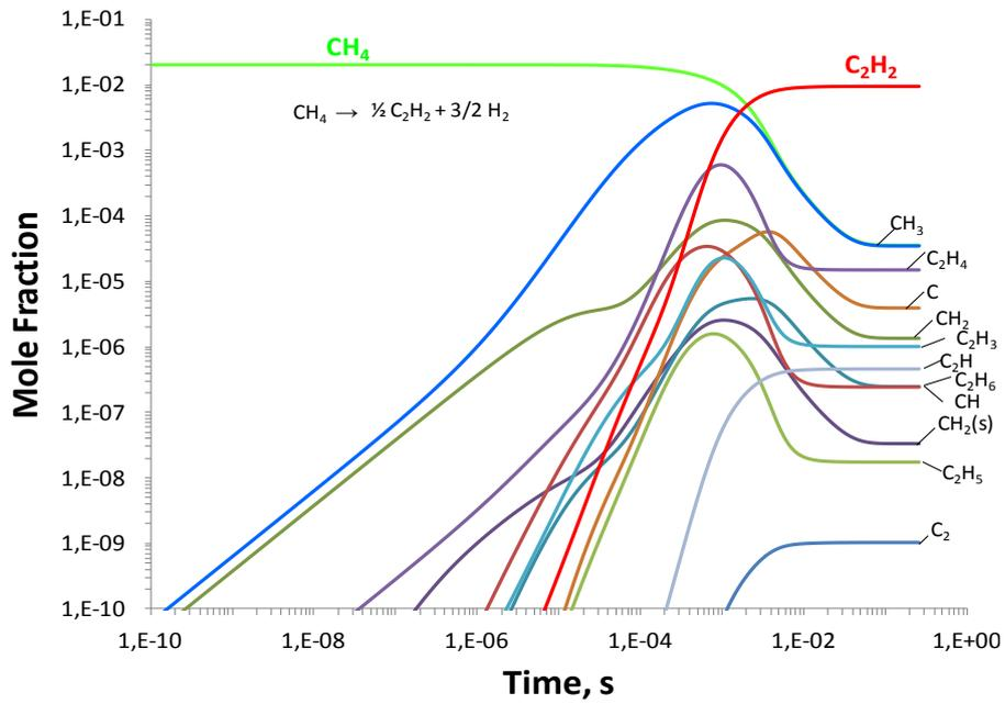
**Figure 11.** Time evolution of small C<sub>1</sub>-C<sub>2</sub> carbon species mole fractions calculated from Table 3, OPT 1 conditions. Global reaction transforming input methane to acetylene. Ts=700°C, P=13 mbar, Φ<sub>CH<sub>4</sub></sub>=1 sccm, Φ<sub>H<sub>2</sub></sub>=50 sccm and P<sub>mw</sub>=400 W.
