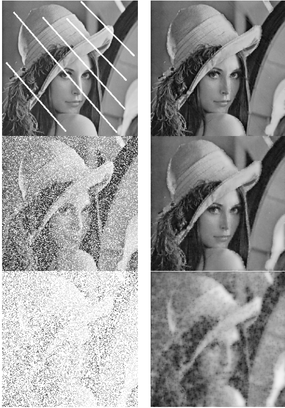
Fig. 4: Three reconstructions via the the varying coefficients restoration procedure: with small diagonal corruptions, and with 30% and 80% of pixels randomly removed.
