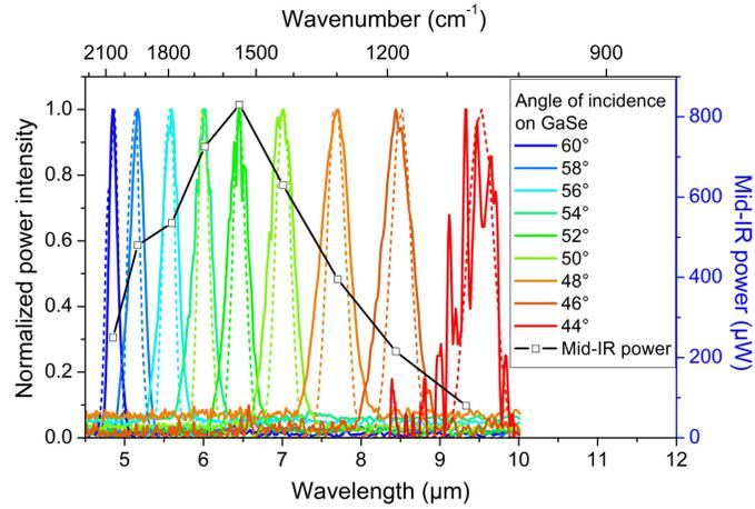
Fig. 7. The mid-IR idler spectra are tunable between  $4.85$  and  $9.33 \text{ }\mu\text{m}$ . The solid lines correspond to the experimental results. The dashed lines depict spectra from a numerical simulation. We used a  $2 \text{ mm}$  long GaSe crystal.
