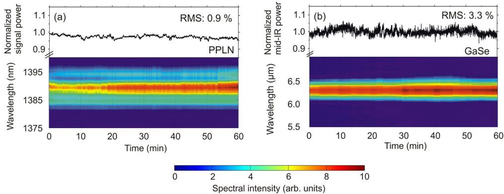
Fig. 8. Temporal stability of power and spectra (a) in the near-IR region using a  $5 \text{ mm}$  PPLN crystal and (b) in the mid-IR region using a  $1 \text{ mm}$  GaSe crystal. All measurements were performed over one hour.
