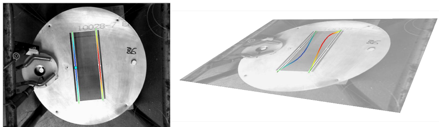
Figure 6. Experimental mode shape for the out-of phase mode (top view and 3D view), only the velocity amplitude of the beams have been depicted
