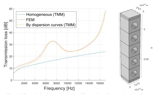
Figure 8: Transmission loss computed for a 3D repetition of 5 melamine unit cells.
