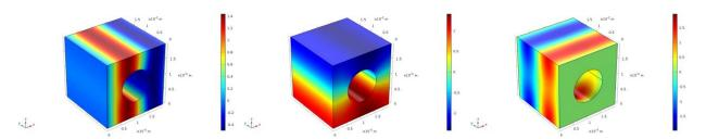
Figure 7: From left to right, real parts of the 1st, 2nd and 3rd branch eigenvectors for the case with an inclusion.
