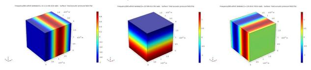
Figure 5: From left to right, real parts of the 1st, 2nd and 3rd branch eigenvectors for the homogeneous case.
