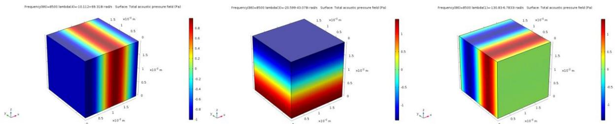
Figure 5: From left to right, real parts of the 1st, 2nd and 3rd branch eigenvectors for the homogeneous case.
