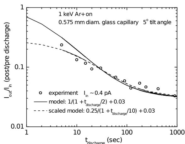
**Figure 1.** – Transmitted intensity as a function of the discharge time, normalized to the transmitted one, just before the beam was blocked, for a cylindrical capillary of 43 mm length, 0.575 mm inner diameter.
