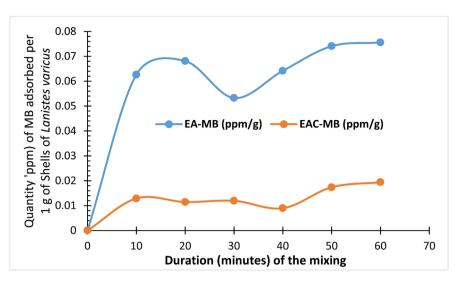
**Figure 20.** Quantities of BM fixed on *Lanistes varicus* shells as function of the duration of the mixing.
