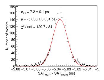
Figure 4: Difference of the signal arrival times at the two MCP-PMTs. Data are selected by requiring a particle track passing through the inner 11 mm of the first MCP. A combined time resolution of  $(7.2\pm0.1)$  ps is measured from a Gaussian fit (red line).
