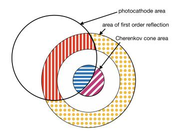
Figure 2: Sketch of the geometrical overlap between Cherenkov cone, in blue horizontal hatching and violet diagonal hatching, and first-order reflected light, in red vertical hatching and yellow dotted shaded areas, with the photocathode area, as a thick black line.
