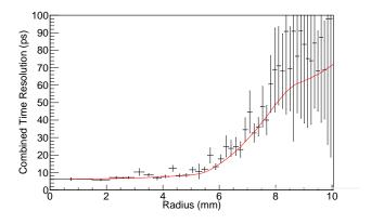
Figure 5: Combined time resolution as a function of the track impact point distance from the photocathode center. The red line shows a possible modelling using results from the Monte-Carlo simulation, as explained in Sec. 2.
