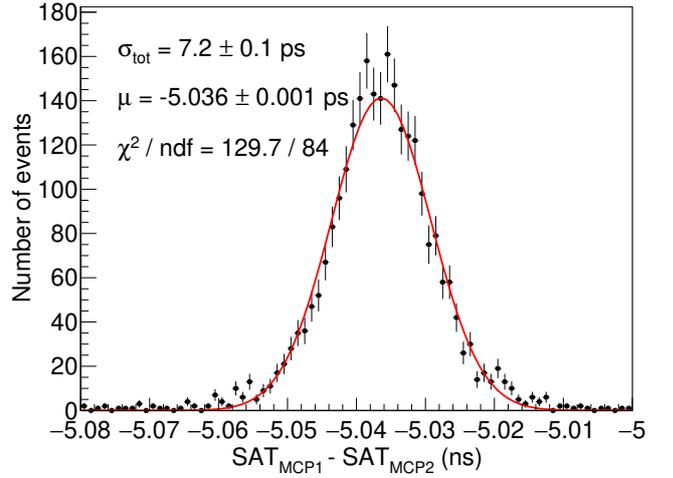
Figure 4: Difference of the signal arrival times at the two MCP-PMTs. Data are selected by requiring a particle track passing through the inner 11 mm of the first MCP. A combined time resolution of  $(7.2 \pm 0.1)$  ps is measured from a Gaussian fit (red line).
