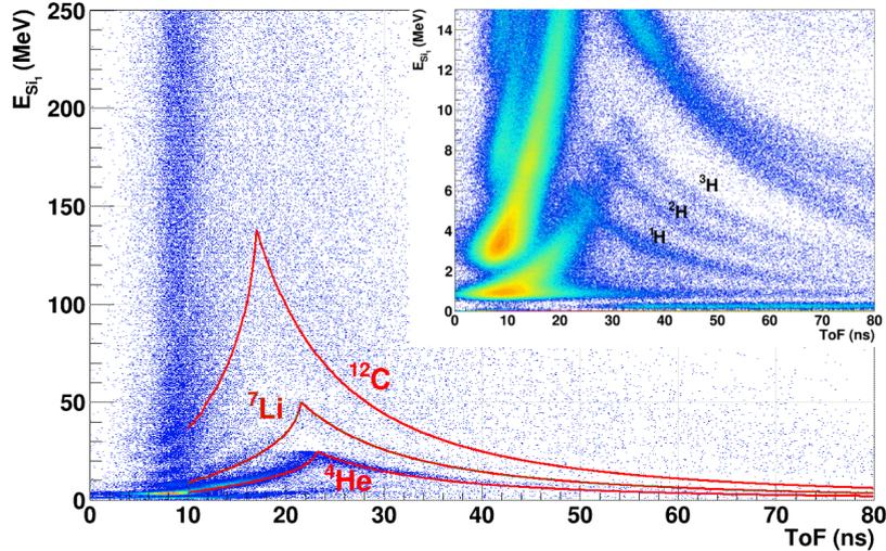
Fig. 2. –  $E - ToF$  correlation for a typical first layer silicon detector during the first FAZIA experiment. Only Hydrogen isotopes are resolved.
