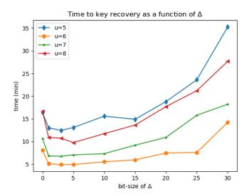
Fig. 1: Analyzing the overall time to recover the secret key as a function of the bitsize of  $\Delta$ . We report the numbers BKZ-25 and no preprocessing. The optimal value for  $\Delta$  is around  $2^3$  except for u=8 where it is  $2^5$ .
