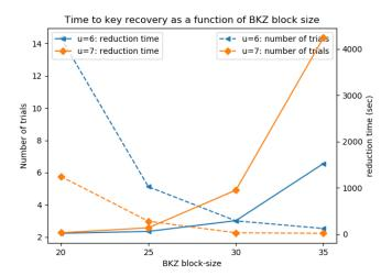
Fig. 3: Analyzing the number of trials to recover the secret key and the reduction time of the lattice as a function of the block-size of BKZ. We consider the cases where u = 6 and u = 7. The dotted lines correspond to the number of trials, and the continued lines to the reduction time in seconds.
