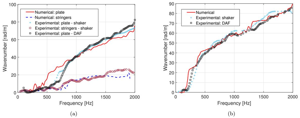
Figure 18: Dispersion curves for the bare configuration and different loading conditions: axial (a) and circumferential (b) directions
