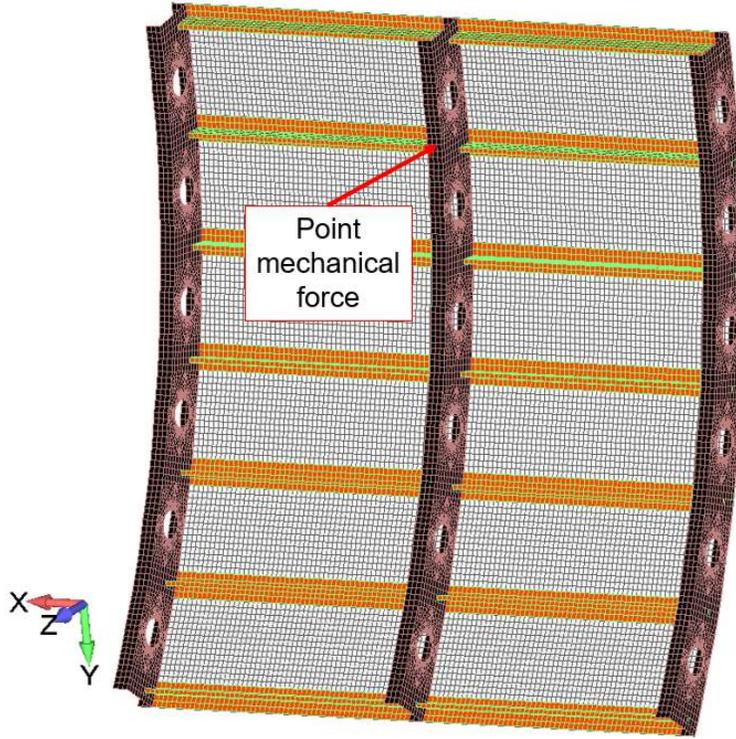
Figure 17: Finite element model of the aluminum panel
