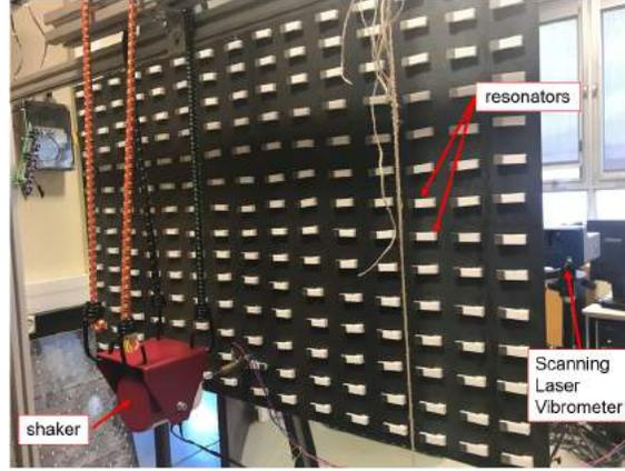
Figure 4: Set-up of the steel plate with distributed resonators
