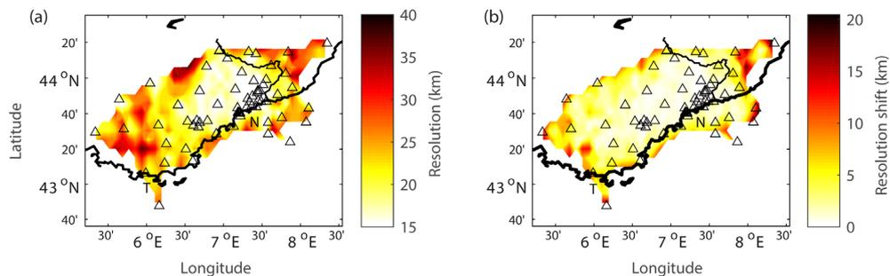
**Figure 9.** (a) Spatial resolution map for Rayleigh waves at 4 s. (b) Resolution shift map for Rayleigh wave at 4 s. For the two figures, the black bold curve shows the coastline. Seismic stations are shown as black outline triangles. The black bold curve shows the coastline. The thinner black curve indicates the Franco–Italian border.
