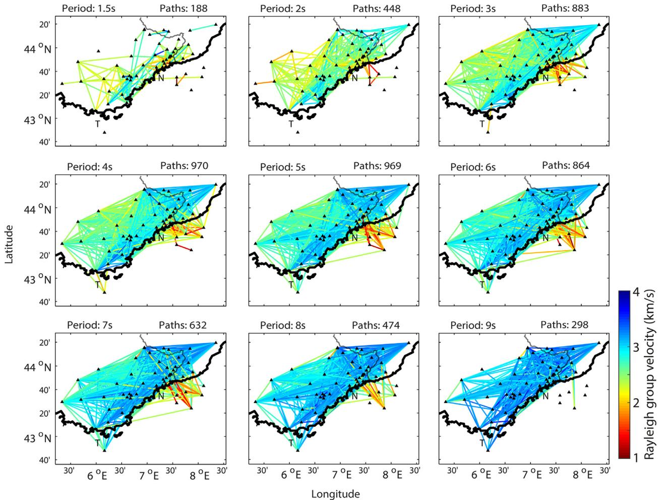
**Figure 6.** Rayleigh-wave group velocity measurements for ZZ components and associated ray path coverage to periods from 1.5 to 9 s. Seismic stations are shown as black triangles. T indicates the city of Toulon. N indicates the city of Nice. Grey curve shows the Franco-Italian border.
