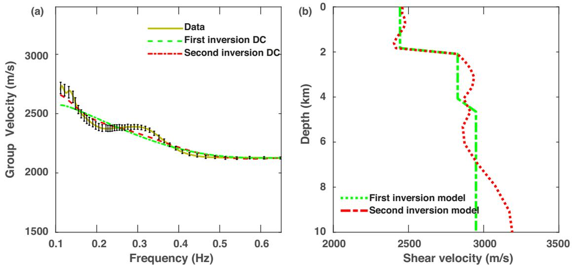
**Figure 11.** (a) Group velocity dispersion curves for the cell below the city of Nice: data from dispersion measurement (yellow), synthetic DC from the three-layer model (green), and from the multilayer model (red). (b) Shear velocity depth models using group velocities: initial three-layer model (green) and final multilayer model (red). The black error bar is computed the same way as the first inversion but divided by a factor of 2. chi-squared is less than 0.5 for this cell.
