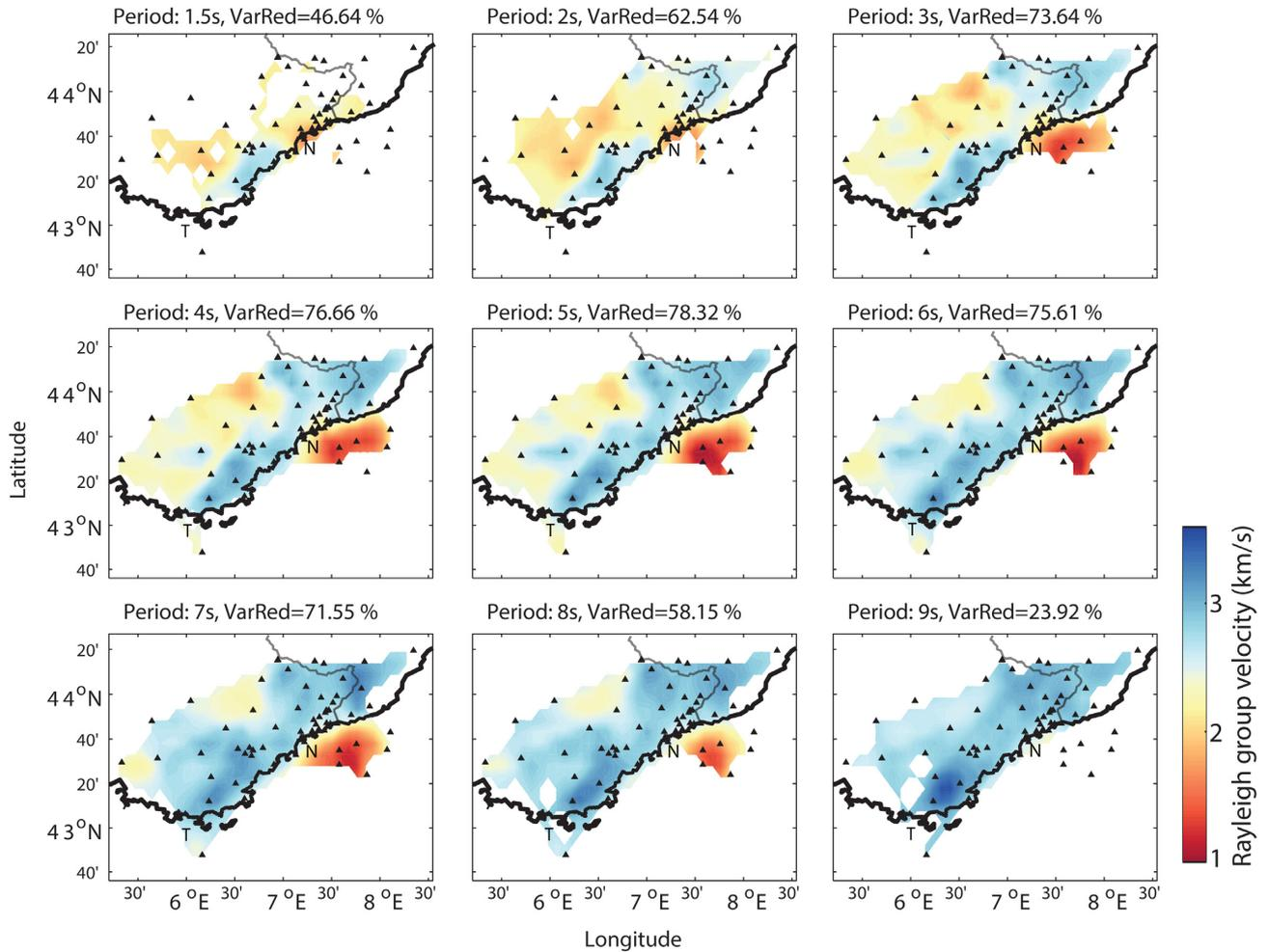
**Figure 7.** Rayleigh and Scholte wave group-velocity maps for 1.5, 2, 3, 4, 5, 6, 7, 8 and 9 s, respectively. At each period, we indicated the variance reduction (VarRed) between data computed from the measurement and the final model. The black bold curve shows the coastline while the grey curve indicates the Franco–Italian border. Seismic stations are shown as black triangles. T indicates the city of Toulon. N indicates the city of Nice.
