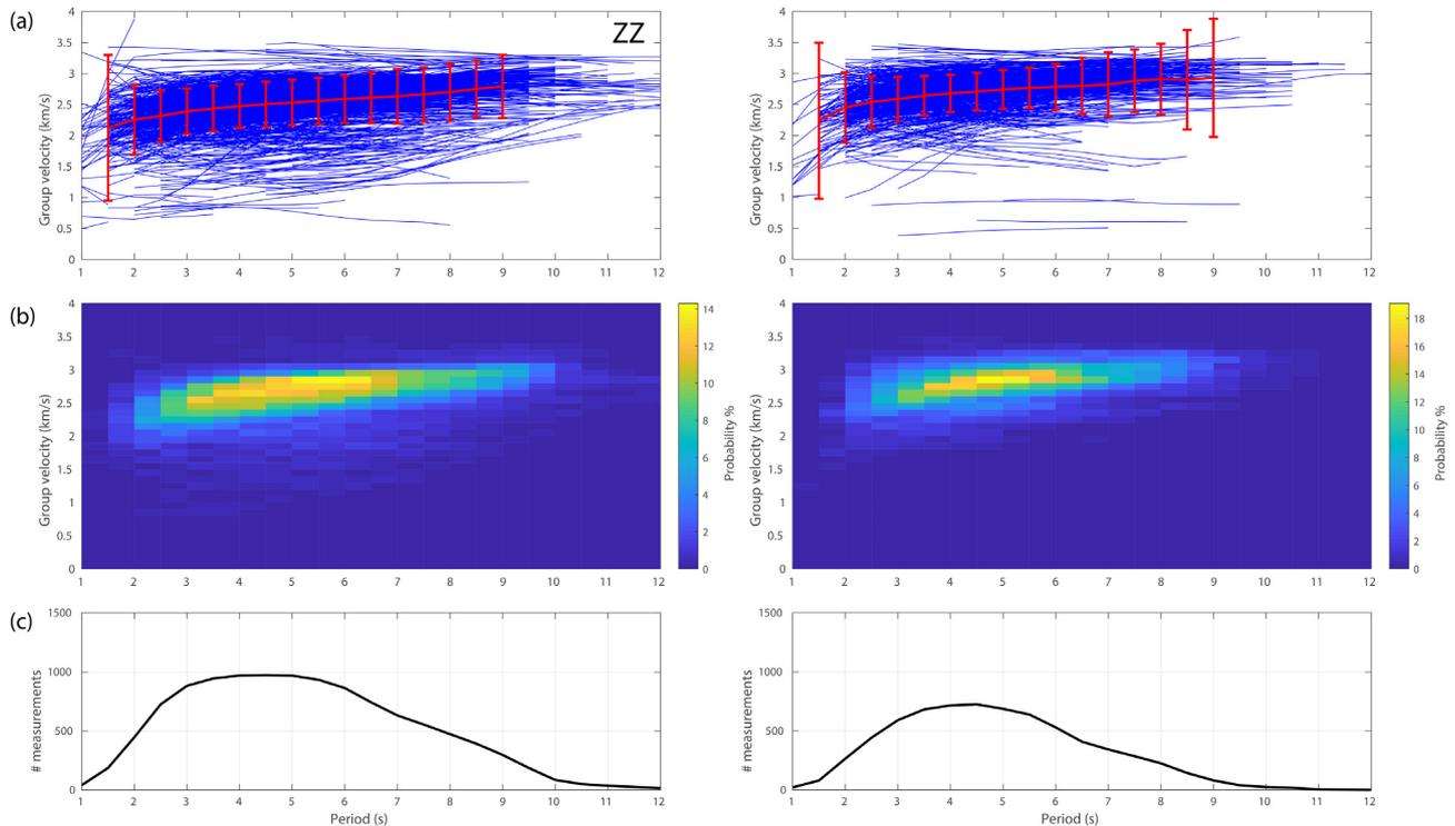
**Figure 5.** (a) All measured Rayleigh and Love-wave dispersion curves are plotted on a group velocity–period diagram. The average dispersion curve with its standard deviation is plotted as red line and only for periods ranging from 1.5 to 9 s which are the periods shown on group velocity maps (b) Probability density diagram of the dispersion curves. (c) Diagram representing the number of measurements with respect to period for ZZ (left-hand panel) and TT (right-hand panel).
