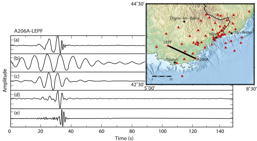
**Figure 3.** Cross-correlation between A206A-LEPF filtered for several labelled period bands and computed for the ZZ components of ambient noise. (a) Broad-band signal (0.4–14 s passband), while filtered signal is shown below with (b) 8–10 s, (c) 5–8 s, (d) 2–5 s and (e) 0.4–2 s. Black curve on the map indicates the path A206A-LEPF. Inter stations distance is 80 km.
