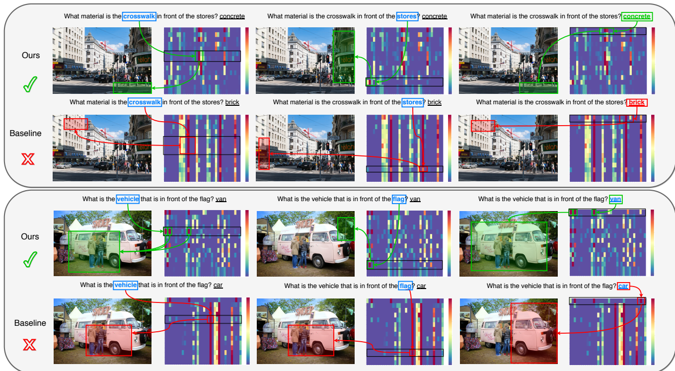
Figure 4. Visualization of the attention maps of the penultimate (=4th) inter-modality transformer. Word-object alignment does not emerge naturally for the baseline (without object-word alignment supervision), whereas our model with the proposed weakly-supervised objective learns to pay strong cross-attention on co-occurring combinations of words and objects in the scene. In the attention maps, rows represent words and columns represent visual objects. For the sake of visibility, we display the bounding box of the detected object with the highest activation regarding to the selected word. The predicted answer (underlined) is written after the question. Its corresponding language token is [CLS] , i.e., the first row in attention maps.
