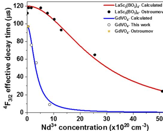
**Fig. 4.** Effective luminescence-decay time measured in  $\text{LaSc}_3(\text{BO}_3)_4$  (black circles [11]) and  $\text{GdVO}_4$  (white circles [present work]; yellow star [11]) as a function of  $\text{Nd}^{3+}$  concentration. The corresponding fits calculated according to Eqs. (6) and (7) are also included (red line for  $\text{LaSc}_3(\text{BO}_3)_4$ , blue line for  $\text{GdVO}_4$ ).
