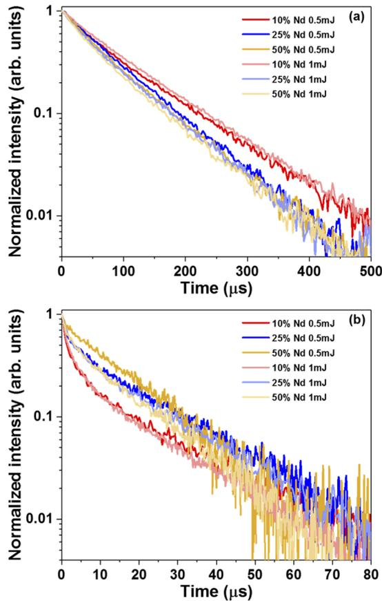
**Fig. 3.** Luminescence transients of (a) infrared luminescence from the  ${}^4\text{F}_{3/2}$  level and (b) visible upconversion luminescence from the  ${}^4\text{G}_{7/2}$  level of  $\text{Nd}^{3+}$  in  $\text{LaSc}_3(\text{BO}_3)_4$  crystals with three different  $\text{Nd}^{3+}$  concentrations and two different pump energies.
