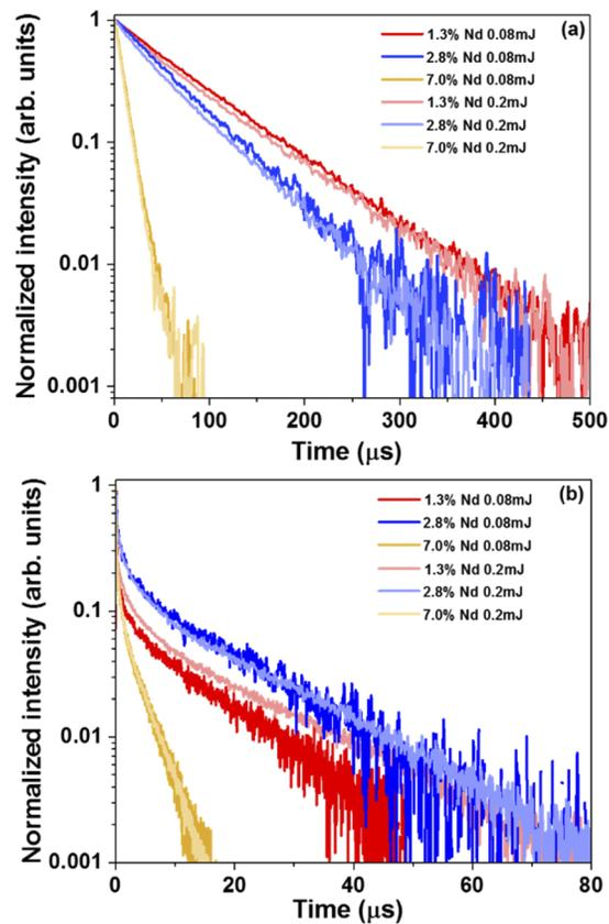
**Fig. 2.** Luminescence transients of (a) infrared luminescence from the  $^4\text{F}_{3/2}$  level and (b) visible upconversion luminescence from the  $^4\text{G}_{7/2}$  level of  $\text{Nd}^{3+}$  in  $\text{GdVO}_4$  crystals with three different  $\text{Nd}^{3+}$  concentrations and two different pump energies.
