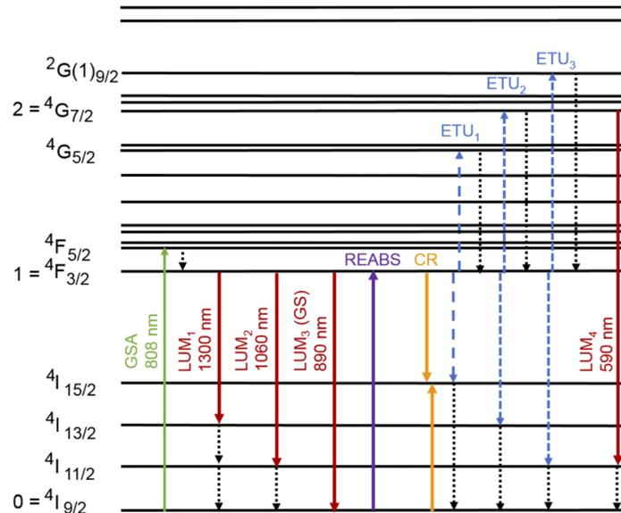
**Fig. 1.** Partial energy-level diagram of  $\text{Nd}^{3+}$  indicating the relevant spectroscopic processes: ground-state absorption (GSA), luminescence decay (LUM), reabsorption (REABS), cross relaxation (CR), energy-transfer upconversion (ETU), and multiphonon relaxation (dotted arrows). The levels considered for the simplified three-level scheme are numbered on the left-hand side.
