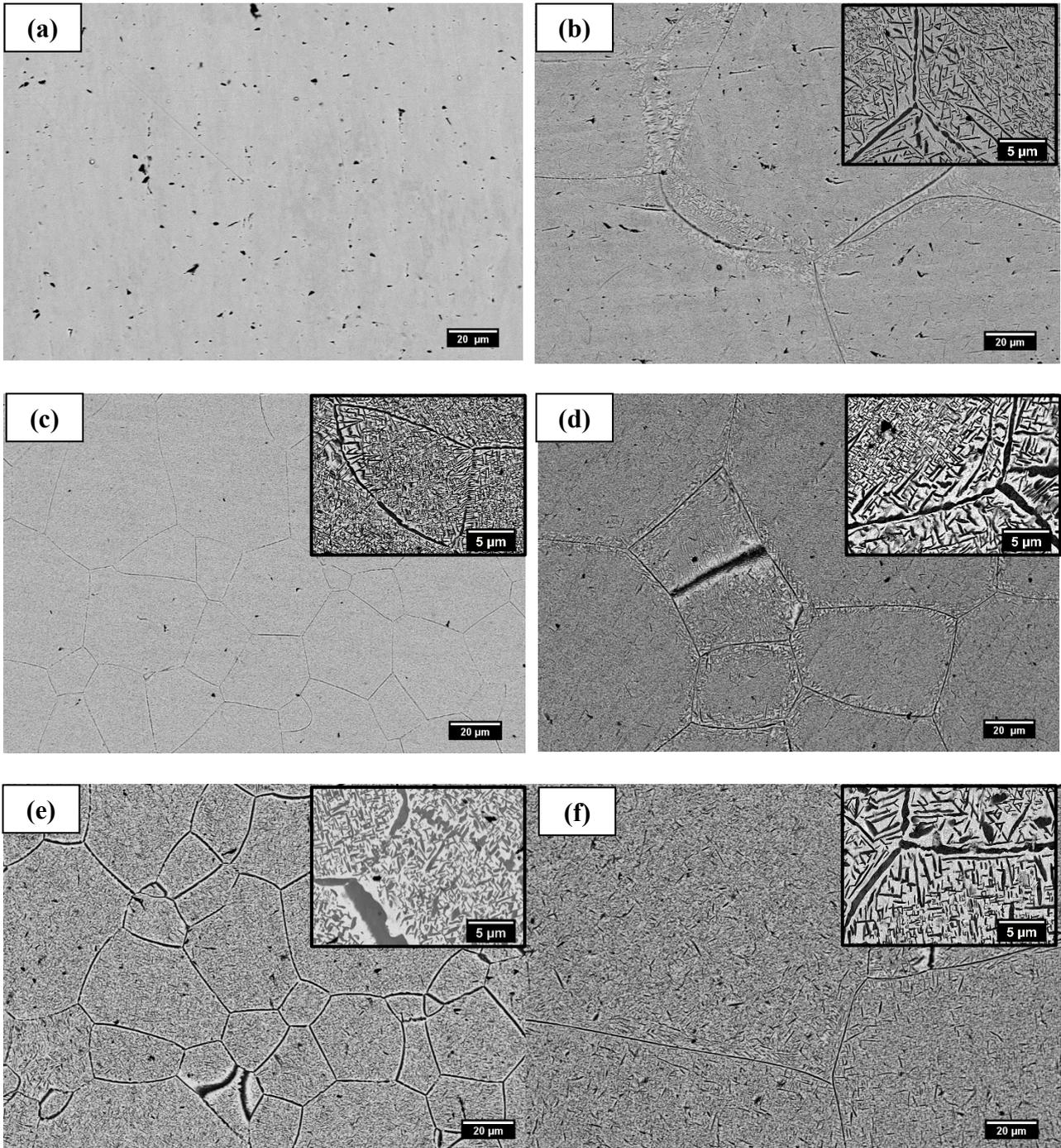
Fig 1: Microstructure observations of Ti- $\beta$ 21S for the two types of specimen used: as-received solution treatment (left column) and precipitation treatment (right column). The images shown correspond to the initial state (a,b), after thermal aging for 500 h at 600°C (c,d) and 650°C (e,f).
