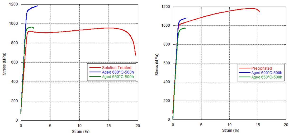
Fig 2: Tensile true-stress-true-strain curves for the solution (left plot) and the precipitated (right plot) microstructures.
