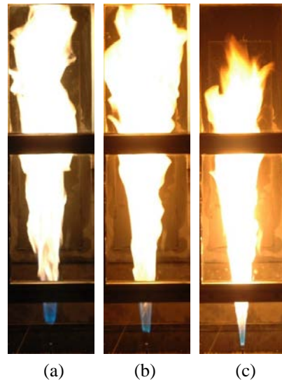
Fig. 1. Flame photographs, (a) mb = 0.3 , (b) mb/e = 70/30 , (c) me = 0.166 . Exposure = 1/20 s. Images are 645 mm in height.
