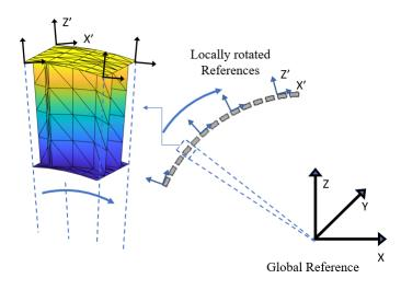
Figure 2: Example of a FE cell curved rotating the local nodal references.
