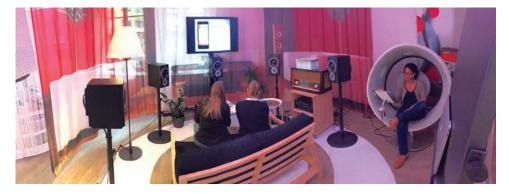
Fig. 5. ORPHEUS test installation at *open innovation lab* JOSEPHS; left side: loudspeaker reproduction at home; right side: headphone reproduction in a noisy environment (produced by loudspeakers in sonic chair), *mobile listening*.
