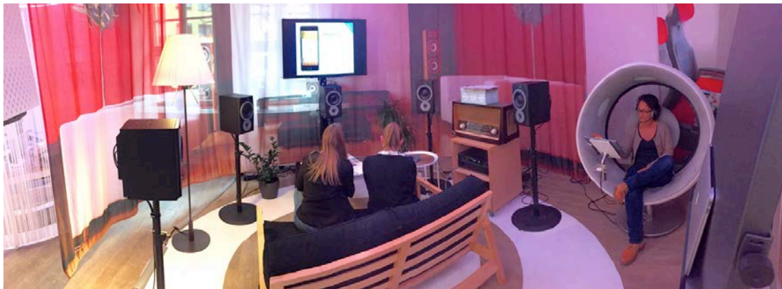
Figure 2: ORPHEUS test installation at open innovation lab JOSEPHS; left side: loudspeaker reproduction 'at home'; right side: headphone reproduction in a noise environment (produced by loudspeakers in sonic chair) 'on-the go'.
