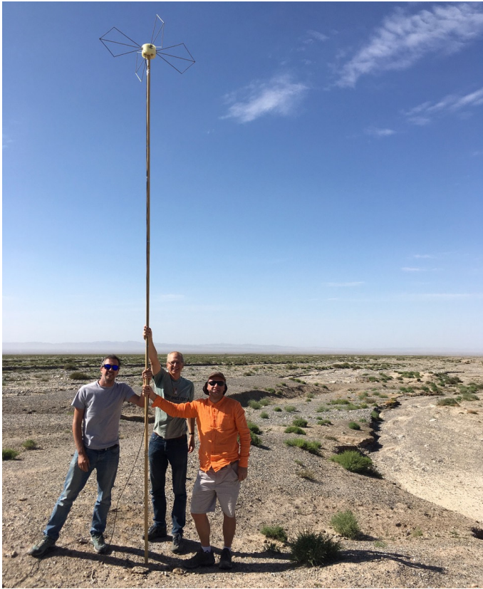
FIG. 33. A prototype of the HORIZONANTENNA in test during a GRANDProto300 site survey. Photo by Feng Yang.
