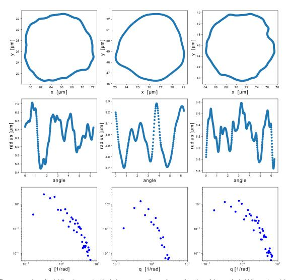
**Fig. S1.** Three examples of wrinkling (top row) with their corresponding radius as function of the angle (middle row) and their Fourier spectrum (bottom row). The maximal value of the Fourier spectrum is selected as characteristic wavelength.
