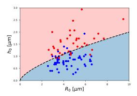
**Fig. 3.** Buckled (blue dots) and wrinkled (red dots) shapes plotted in a  $(h_0, R_0)$  diagram. The dashed line is the best fit of data points with Eq. 5 and separates regions where buckling (blue) or wrinkling (pink) occurs.
