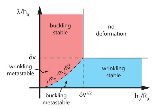
**Fig. S3.** Stability diagram of a spherical vesicle with an actin shell undergoing both wrinkling and buckling. The dotted line represents the equality of tension  $\gamma$  for both buckling and wrinkling.
