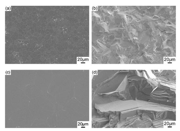
Fig. 21. SEM images of the (a, c) thermally etched and (b, d) freshly fractured surfaces of 5 at%Yb:Sc<sub>2</sub>O<sub>3</sub> ceramics sintered for 10 h at either (a, b) 1650 °C or (c, d) 1850 °C. Reused from [166]. Copyright © 2017, Elsevier.
