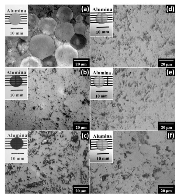
Fig. 12. SEM images and photographs of the Al<sub>2</sub>O<sub>3</sub> samples sintered at 5.0 GPa and high temperature: (a–c) coarse powder, (d–f) mixture of coarse powder and nanopowder, (a, d) 5.0 GPa and 700 °C, (b, e) 5.0 GPa and 900 °C, and (c, f) 5.0 GPa and 1100 °C. Reused from [81], Copyright © 2016, Elsevier.
