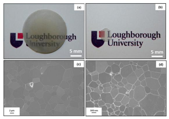
Fig. 6. Photographs and SEM images of transparent  $Al_2O_3$  ceramics prepared under different SPS conditions: (a, c) SPS70-14, (b, d) SPS-500-12. Reused from [72]. Copyright © 2017, Elsevier.
