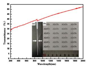
Fig. 11. Transmittance curve of the transparent  $Al_2O_3$  ceramic wafers with a (a) side view photograph and (b) planetary view photograph. Reused from [79], Copyright © 2018, Elsevier.
