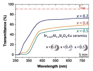
**Fig. 38.** Transmittance curves of 1.1-mm thick samples of the Eu-doped  $Sr_{1-x/}$   $_2Al_{2-x}Si_xO_4$  (x=0.2, 0.4,and 0.5) ceramics. Reused from [399], Copyright © 2017, American Chemical Society.
