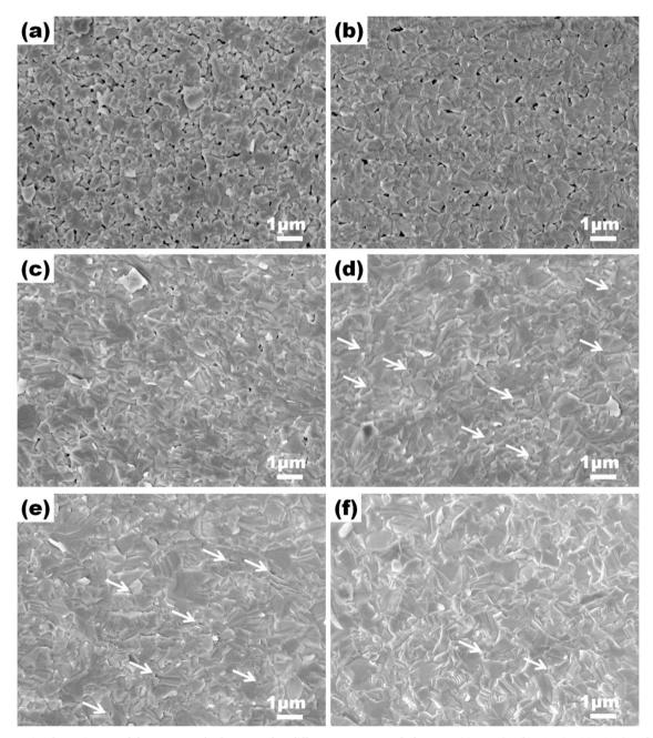
Fig. 18. Cross-sectional SEM images of the  $Y_2O_3$  samples hot-pressed at different temperatures before HIP: (a)  $1300\,^{\circ}$ C, (b)  $1350\,^{\circ}$ C, (c)  $1400\,^{\circ}$ C, (d)  $1450\,^{\circ}$ C, (e)  $1500\,^{\circ}$ C, and (f)  $1550\,^{\circ}$ C. Reused from [143]. Copyright © 2018, Elsevier.
