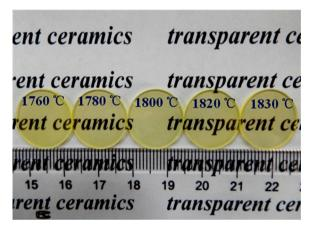
Fig. 29. Photographs of polished DyAG ceramics,  $\phi16\,\text{mm}\times1\,\text{mm}$ , sintered at different temperatures. Reused from [261], Copyright © 2015, John Wiley & Sons
