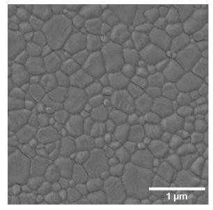
Fig. 2. Representative SEM image of  ${\rm Er}^{3+}$ -doped  ${\rm Al}_2{\rm O}_3$  ceramics after HIP. Reused from [61]. Copyright © 2017, Elsevier.
