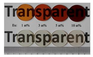
**Fig. 35.** Photographs of the as-sintered (above) and thermally annealed (below)  $\mathrm{Eu}^{3+}$ -doped  $\mathrm{La}_{0.8}\mathrm{Gd}_{1.2}\mathrm{Hf}_2\mathrm{O}_7$  ceramics. Reused from [394], Copyright © 2017, Elsevier.
