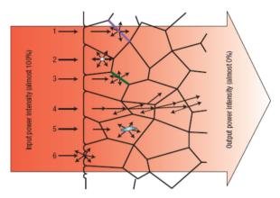
**Fig. 1.** Possible sources of light scattering in ceramics: (1) grain boundaries, (2) pores, (3) impurities, (4) double refraction, (5) secondary phase, and (6) surface roughness. Reused from [2], Copyright © 2008, Nature Publishing Group.
