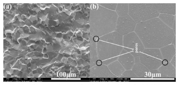
Fig. 10. Representative SEM images of the transparent  $Al_2O_3$  ceramic wafers: (a) fracture surface and (b) thermally etched polished surface. Reused from [79], Copyright © 2018, Elsevier.
