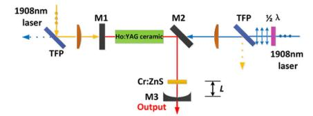
Fig. 45. Schematic diagram of the high-power dual-end-pumped passively Q-switched Ho:YAG ceramic laser experimental setup. Reused from [566], Copyright © 2015, Springer.
