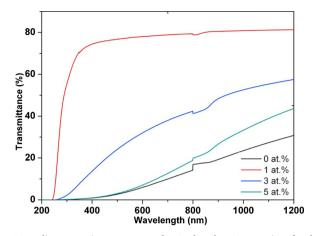
Fig. 15. In-line transmittance curves of  $ZrO_2$ -doped  $Y_2O_3$  ceramics after hot-pressing at  $1600\,^{\circ}C$  and  $20\,MPa$  for  $3\,h$ . Reproduced from [123]. Copyright © 2017, Elsevier.
