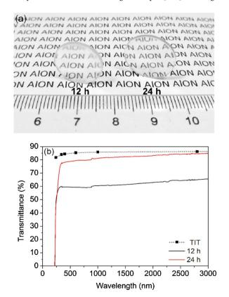
Fig. 40. (a) Photographs and (b) in-line transmittance curves of 1-mm thick samples of the transparent AlON ceramics derived from powders milled for  $12\,h$  and  $24\,h$  and sintered at  $1850\,^{\circ}\text{C}$  for  $360\,\text{min}$ . Reused from [420], Copyright © 2016, Elsevier.
