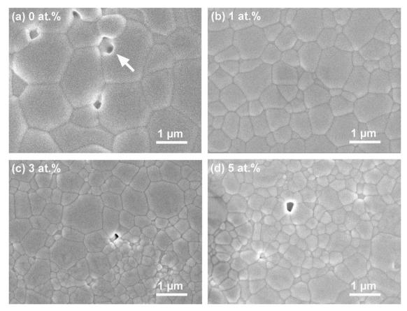
Fig. 16. SEM images of the  $ZrO_2$ -doped  $Y_2O_3$  ceramics after hot-pressing at 1600 °C and 20 MPa for 3 h: (a) 0 at%  $ZrO_2$ , (b) 1 at%  $ZrO_2$ , (c) 3 at%  $ZrO_2$ , and (d) 5 at%  $ZrO_2$ . Reproduced from [123]. Copyright © 2017, Elsevier.
