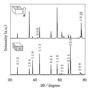
**Fig. 7.** XRD spectra of the planes perpendicular and parallel to the magnetic field; the  $Al_2O_3$  samples were sintered at 1150 °C for 20 min after heating at 2 °C/min. Reused from [73]. Copyright © 2018, Elsevier.
