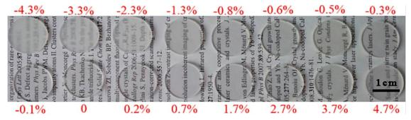
Fig. 23. Photographs of  $\Phi16 \text{ mm} \times 1.5 \text{ mm}$  samples of  $Y_{3(1+x)}Al_5O_{12}$  ceramics with different values of x after sintering at 1760 °C for 10 h. Reused from [211]. Copyright © 2015, Elsevier.
