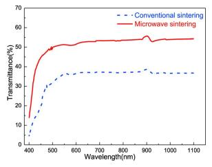
**Fig. 32.** In-line transmittance curves of PLZT ceramics (0.3-mm thick samples) fabricated by conventional sintering at  $1200\,^{\circ}$ C for 3 h and microwave sintering at  $1000\,^{\circ}$ C for 20 min. Reused from [335], Copyright © 2017, Elsevier.
