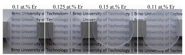
Fig. 4. Photographs of transparent  $Er^{3+}$ -doped  $Al_2O_3$  ceramics with an approximate diameter of 3 cm, positioned 1 cm above the text. Reused from [61]. Copyright © 2017, Elsevier.
