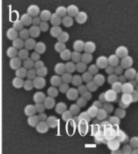
Fig. 22. SEM images of (a) Lu(OH)CO<sub>3</sub> and (b) (Lu<sub>0.95</sub>Eu<sub>0.05</sub>)OHCO<sub>3</sub> precursor powders. Reused from [171]. Copyright © 2015, Elsevier.
