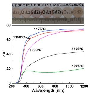
Fig. 37. Photographs and in-line transmittance curves of 1-mm thick samples of the LaGdZr $_2$ O $_7$  ceramics prepared from powders calcined at different temperatures and sintered at 1800 °C for 10 h. Reproduced from [387]. Copyright © 2018, Elsevier.
