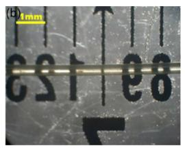
Fig. 33. Photographs of (a) the as-extruded PLZT green fibers and (b) a sintered transparent PLZT ceramic fiber. Reused from [336], @Copyright 2016, Elsevier.
