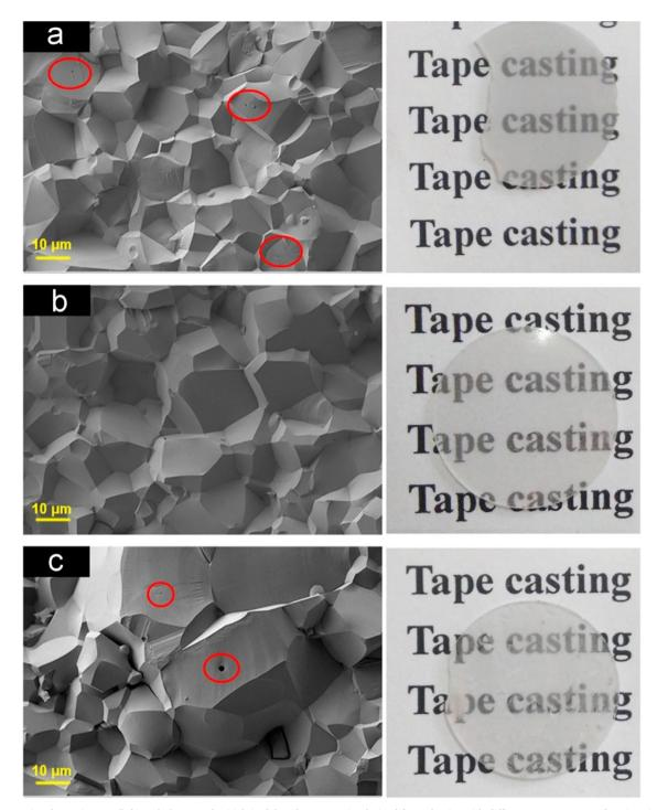
Fig. 8. Cross-sectional SEM images (left) and photographs (right) of the  $Al_2O_3$  ceramics derived from slurries with different PVA contents after sintering at  $1810\,^{\circ}$ C for 5 h: (a) 8 vol%, (b) 10 vol%, and (c) 12 vol%. Reused from [78]. Copyright © 2016, Elsevier.
