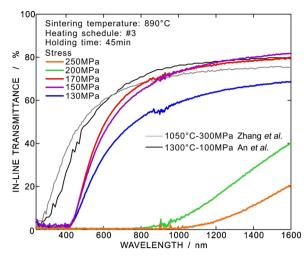
**Fig. 19.** In-line transmittance curves of the  $Y_2O_3$  ceramics sintered at 890 °C for 0.5 h under different loading stresses: (a) 130 MPa, (b) 170 MPa, (c) 200 MPa, and (d) 250 MPa. Literature transmittance data for undoped transparent  $Y_2O_3$  ceramics prepared by SPS at 1050 °C and 300 MPa [144] and 1300 °C and 100 MPa [843] are included for comparison. Reproduced from [142]. Copyright © 2018, Elsevier.
