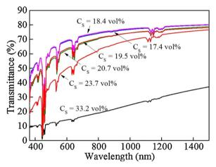
Fig. 20. In-line transmittance curves of 2.14-mm thick samples of the  $\rm ZrO_2$ -doped Ho: $\rm Y_2O_3$  ceramics derived from slurries with different concentrations. Reused from [154]. Copyright © 2015, Elsevier.
