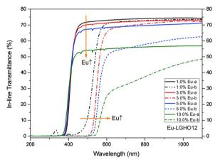
**Fig. 36.** In-line transmittance curves of 1-mm thick samples of the  $\mathrm{Eu}^{3+}$ -doped  $\mathrm{La_{0.8}Gd_{1.2}Hf_2O_7}$  ceramics: (a) annealed (solid lines) and (b) unannealed (dash lines). Reused from [394], Copyright © 2017, Elsevier.
