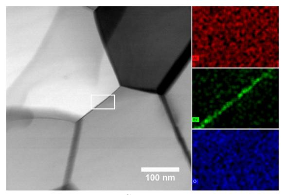
Fig. 3. TEM image and EDS profiles (Al, Er, O) of the 0.1 at% Er<sup>3+</sup>-doped Al<sub>2</sub>O<sub>3</sub> grain boundary. Reused from [61]. Copyright © 2017, Elsevier.
