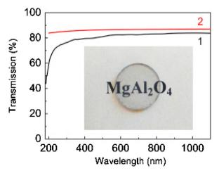
Fig. 30. Experimental (1) and calculated (2) transmission spectra of 1-mm thick transparent  $MgAl_2O_4$  ceramics doped with 3 wt% LiF. Inset shows a photograph of the experimental sample. Reused from [293], Copyright © 2015, Elsevier.
