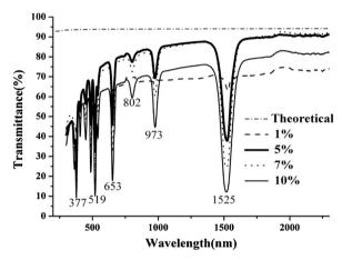
Fig. 43. Photograph and in-line transmittance curves of 2-mm thick samples of the transparent  $CaF_2$  ceramics doped with different concentrations of Er and sintered at 800 °C for 2 h. Reused from [449], Copyright © 2015, Elsevier.
