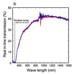
Fig. 41. (a) Photograph of the  $c\text{-Si}_3N_4$  ceramics fabricated at 15.6 GPa and 1800 °C; the division of the ruler is 1 mm and sample thickness is 0.464 mm. (b) Real inline transmittance curves of two representative  $c\text{-Si}_3N_4$  ceramic samples (red and blue lines). Reused from [440], Copyright © 2017, Nature Publishing Group (For interpretation of the references to colour in this figure legend, the reader is referred to the web version of this article).
