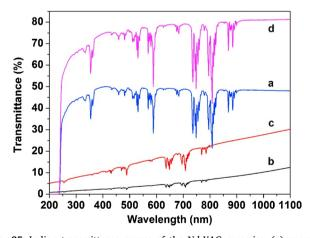
Fig. 25. In-line transmittance curves of the Nd-YAG ceramics: (a) vacuum-sintered at 1800 °C without HIP, (b) vacuum-sintered at 1600 °C followed by HIP at 1600 °C for 3 h, (c) vacuum-sintered at 1700 °C followed by HIP at 1600 °C for 3 h, and (d) vacuum-sintered at 1800 °C followed by HIP at 1600 °C for 3 h. Reused from [218]. Copyright © 2017, Elsevier.
