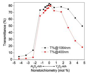
**Fig. 24.** In-line transmission curves of  $\Phi 16\,\text{mm} \times 1.5\,\text{mm}$  samples of non-stoichiometric  $Y_{3(1+x)}Al_5O_{12}$  ceramics after sintering at 1760 °C for 10 h. Reused from [211]. Copyright © 2015, Elsevier.
