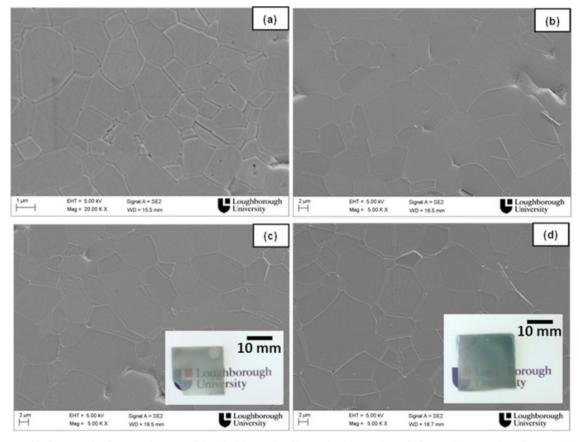
Fig. 5. SEM images of  $Al_2O_3$  samples that were hot pressed for 5 h: (a) 1400 °C, (b) 1500 °C, (c) 1600 °C, and (d) 1700 °C. Insets show the respective photographs. Reused from [72]. Copyright © 2017, Elsevier.
