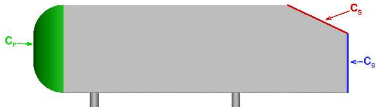
Figure 14: Representation of the pressure drag breakdown.
