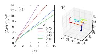
FIG. 2: (a) Mean squared displacement of the center of the vacancies for the hard-cube system at different packing fractions. (b) Trajectory of the center of a vacancy in the hard-cube system at a packing fraction  $\phi = 0.65$ .
