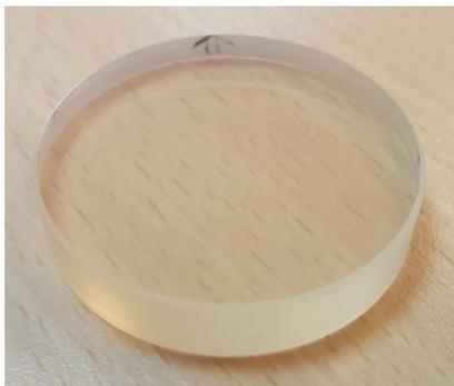
Figure 3. Photo of the manufactured material standard
