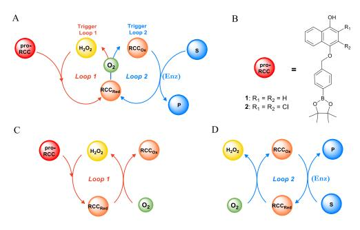
**Scheme 1.** (A) Principle of the  $H_2O_2$ -mediated autocatalytic deprotection of pro-RCC to RCC in the presence of  $O_2$  and a reducing substrate S, the reaction with S being possibly catalysed by an enzyme Enz. (B) Boronate-based probes (pro-RCC) used in this work. (C) Principle of the  $H_2O_2$ -mediated catalytic deprotection of pro-RCC to RCC. (D) Principle of the redox cycling of RCC.
