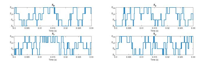
Fig. 10. Switching states for each commutation cell
