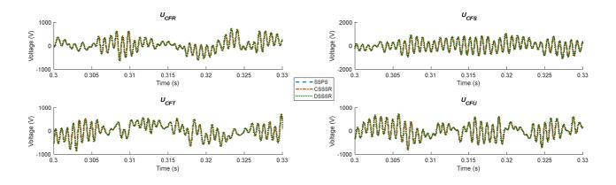
Fig. 7. Voltages across the terminal of the grid filter capacitors
