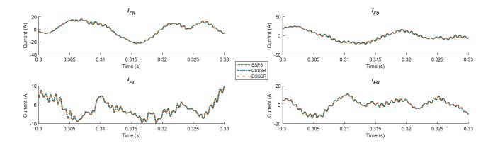
Fig. 6. Currents flowing through the  $L_{Fi}$  inductances of the grid filter
