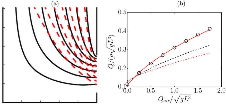
FIG. 8 – Continuum numerical simulation for a silo with a lateral orifice with  $D = 0.40625L$  and  $W = 0.25L$ : (a) Streamlines for the granular flow (red dashed line) and for the air flow (black lines). (b)  $Q/(\rho\sqrt{gL^3})$  as a function of  $Q_{air}/\sqrt{gL^3}$ . The lines represent equation 23 with  $A = 1$  and  $\lambda = 1$  (---),  $A = 0.67$  and  $\lambda = 1$  (---),  $A = 0.67$  and  $\lambda = 0.36$  (-).
