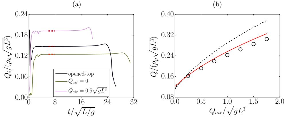
FIG. 4 – Continuum simulation of the discharge of a silo with orifice at the bottom for  $L = 90d$ ,  $D = 0.25L$  and  $W = 0.25L$ : (a) temporal evolution of the dimensionless instantaneous flow rate  $Q_i / (\rho \sqrt{gL^3})$  as a function of the dimensionless time  $t / \sqrt{L/g}$ , (b)  $Q / \rho \sqrt{gL^3}$  as a function of  $Q_{air} / \sqrt{gL^3}$ . The lines represent the simple analytical model (equation 23) with  $A = 1$  (black dashed line) and  $A = 0.68$  (red line).
