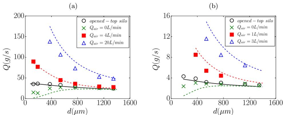
FIG. 9 – Mass flow rate versus size of particles  $d$  for different volume flow rates of air  $Q_{air}$ , for lateral orifices: (a) Cylindrical silo with  $L = 60$  mm,  $D = 20$  mm and  $W = 10$  mm. (b) Rectangular silo with  $L = 60$  mm,  $D = 10$  mm and  $W = 3.5$  mm. The full lines represent Eq. 24 and the dashed lines represent the generalised model 23, with the adjusted parameters given in Table I.
