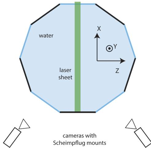
**FIG. 3.** Top view of the stereoscopic optical arrangement used for particle tracking in the LEM flow. Both cameras use an objective with Scheimpflug mount so that all objects in a  $10 \times 10 \times 1 \text{ cm}^3$  region near the geometrical center are approximately in focus on the camera sensor. The calibration mask is placed parallel to the laser sheet and moved in the Z direction.
