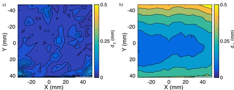
**FIG. 4.** Calibration error averaged over Z using the proposed calibration method (a) or Tsai model (b).
