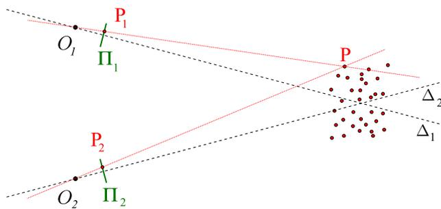
**FIG. 1.** Sketch of Tsai's pinhole camera model and stereo-matching: the position of a particle in the real world corresponds to the intersection of 2 lines  $\Delta_1$  and  $\Delta_2$ , each emitted by the camera centers  $O_1$  and  $O_2$  and passing through the position of particles  $P_1$  and  $P_2$  detected on a each camera plane  $\Pi_1$  and  $\Pi_2$ .
