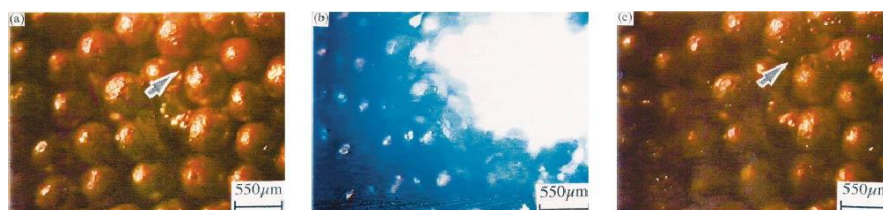
Fig. 10 Image sequence (time interval between each image: 0.02 s) of an electric arc between Cu particles 550 \mu\text{m} in diameter submitted to a single current pulse of 6700 \text{A}/\text{cm}^2 and of 100 ms. Note the welding of the particles (image (c), arrow) resulting from local melting (Yanagisawa et al. 2003).
