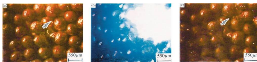
Fig. 10 Image sequence (time interval between each image: 0.02 s) of an electric arc between Cu particles 550 \mu\text{m} in diameter submitted to a single current pulse of 6700 \text{A}/\text{cm}^2 and of 100 ms. Note the welding of the particles (image (c), arrow) resulting from local melting (Yanagisawa et al. 2003).
