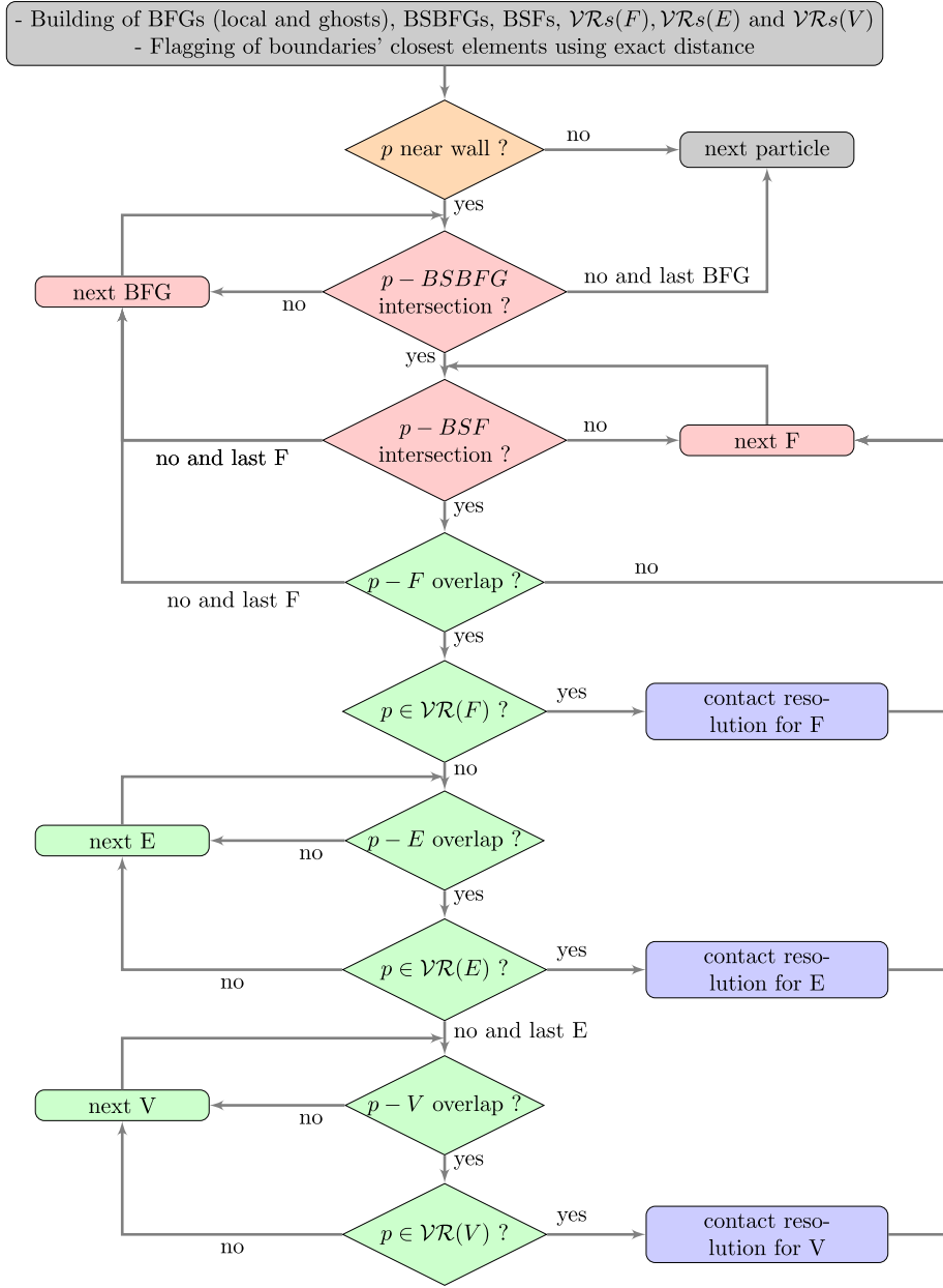
Fig. 21. Flow chart of the definitive procedure followed by each particle for boundary contacts treatment, adapted for arbitrary complex walls. ■ : initializing part and output. ■ : spatial sorting. ■ : null object detector. ■ : contact resolution parts. ■ : \mathcal{VR} tests.
