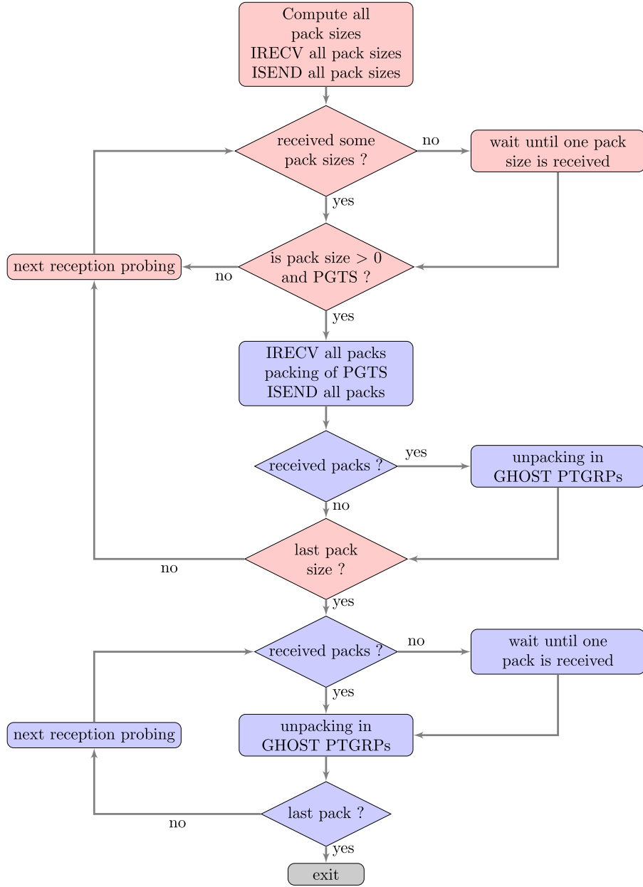
Fig. 12. Flow chart of the final asynchronous algorithm for ghost particle treatment featuring packing/unpacking of the halo data and communication/computation overlap. ■ : pack sizes communication parts. ■ : pack communication parts.
