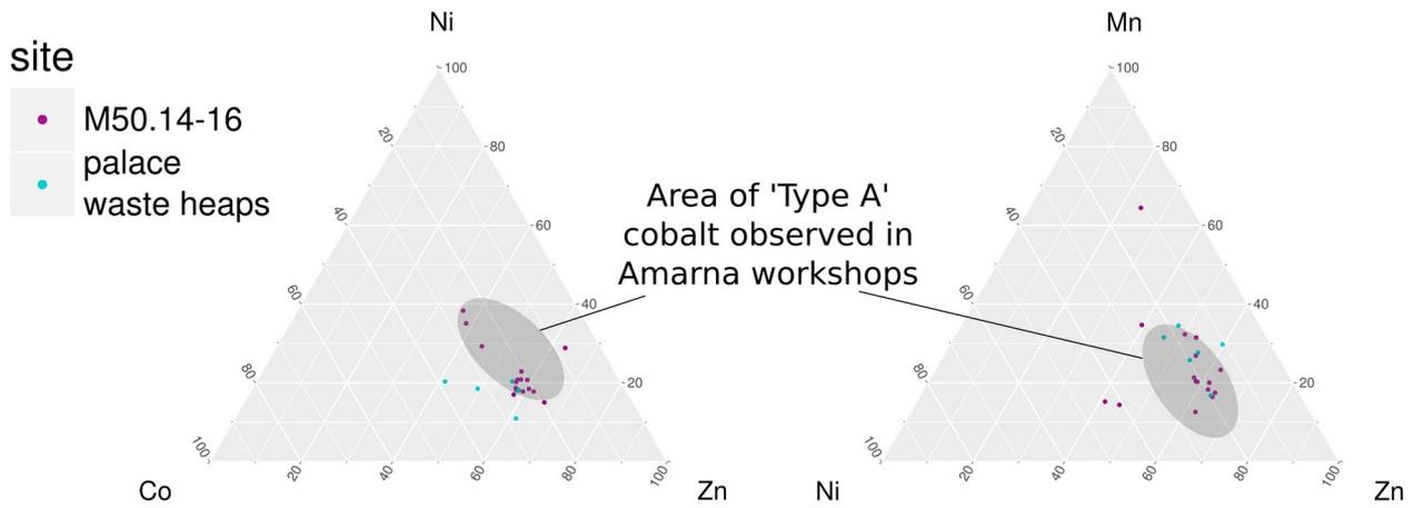
**Figure 10.** Correlation plots showing the Co-Ni-Zn and the Ni-Mn-Zn ratios for cylindrical vessels containing remains of cobalt-blue glass found at Amarna M50.14–16 and the palace waste heaps, as analysed by pXRF. Anna Hodgkinson.
