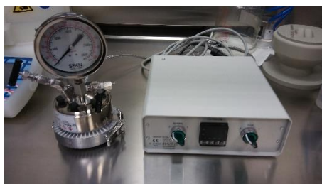
Figure 1. Hydrothermal growth set up with the stainless steel autoclave and temperature regulator.
